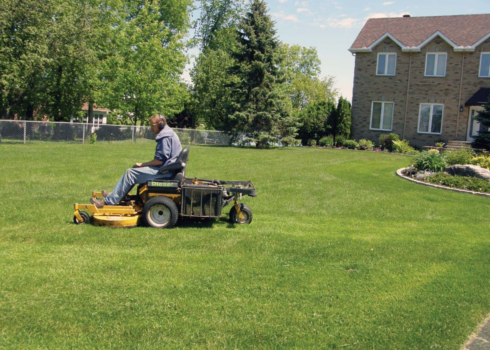
Dave removes the collection hopper during the summer months to reduce weight and lower the mower's center of gravity.
