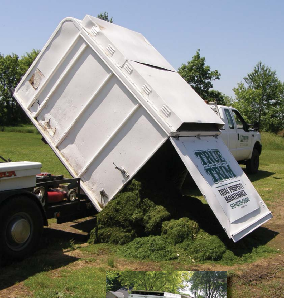
True Trim's owner customized a debris-handling system by fashioning a truck-mounted box to a trailer. When the box is full, the crew hydraulically dumps the debris.
