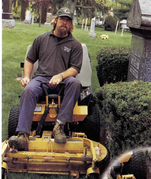
A wear plate protects the mower deck from constant rubbing against headstones.
