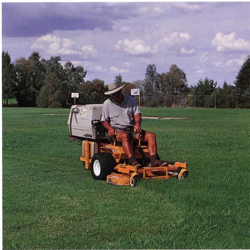
Little’s Mowing Service operates a 21.5-hp diesel Walker with both a grass-handling and side-discharge deck. The setup tackles approximately 16 hectares of grass a week.
