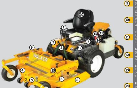
Deck height manually adjusts up to 5" using a foot pedal
