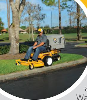
While other mowers use lap bars and arm movements to steer, the Walker uses a forward speed control/cruise control and gentle fingertip pressure on the steering levers to precisely maneuver the machine.
