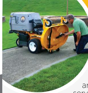
A tilt-open body quickly exposes the engine and drivetrain, while the tilt-up mower deck makes blade maintenance and deck cleaning a quick and easy task.
