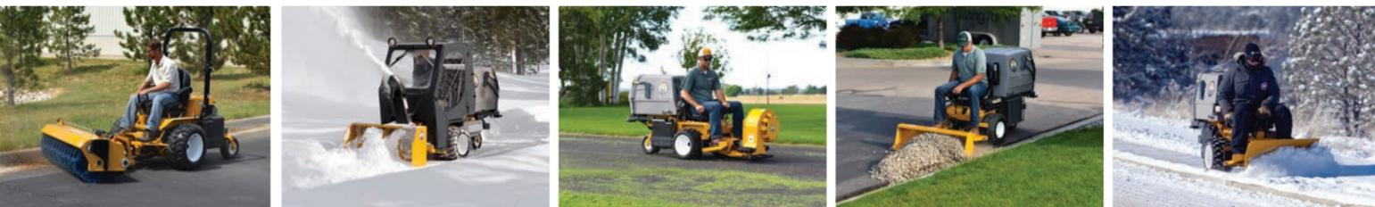
Rotary Broom    Two-Stage Snow Blower    Debris Blower    Loader Bucket    Dozer Blade
