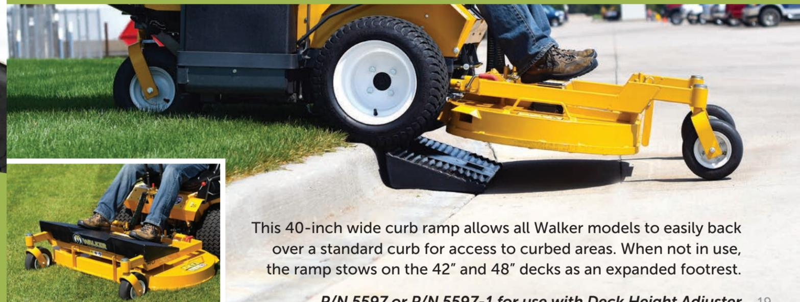
This 40-inch wide curb ramp allows all Walker models to easily back over a standard curb for access to curbed areas. When not in use, the ramp stows on the 42" and 48" decks as an expanded footrest.
