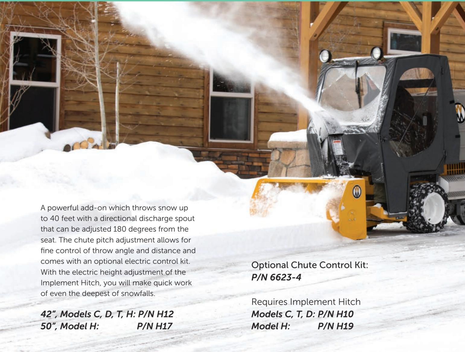
A powerful add-on which throws snow up to 40 feet with a directional discharge spout that can be adjusted 180 degrees from the seat. The chute pitch adjustment allows for fine control of throw angle and distance and comes with an optional electric control kit. With the electric height adjustment of the Implement Hitch, you will make quick work of even the deepest of snowfalls.
