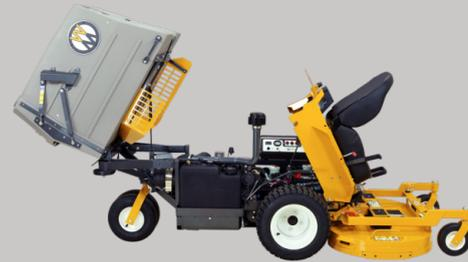
Tilt-open bodies quickly expose engine and drive train for service and easy maintenance.
