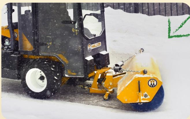
Operator Hard Cab, Implement Hitch, and 60" Rotary Broom
