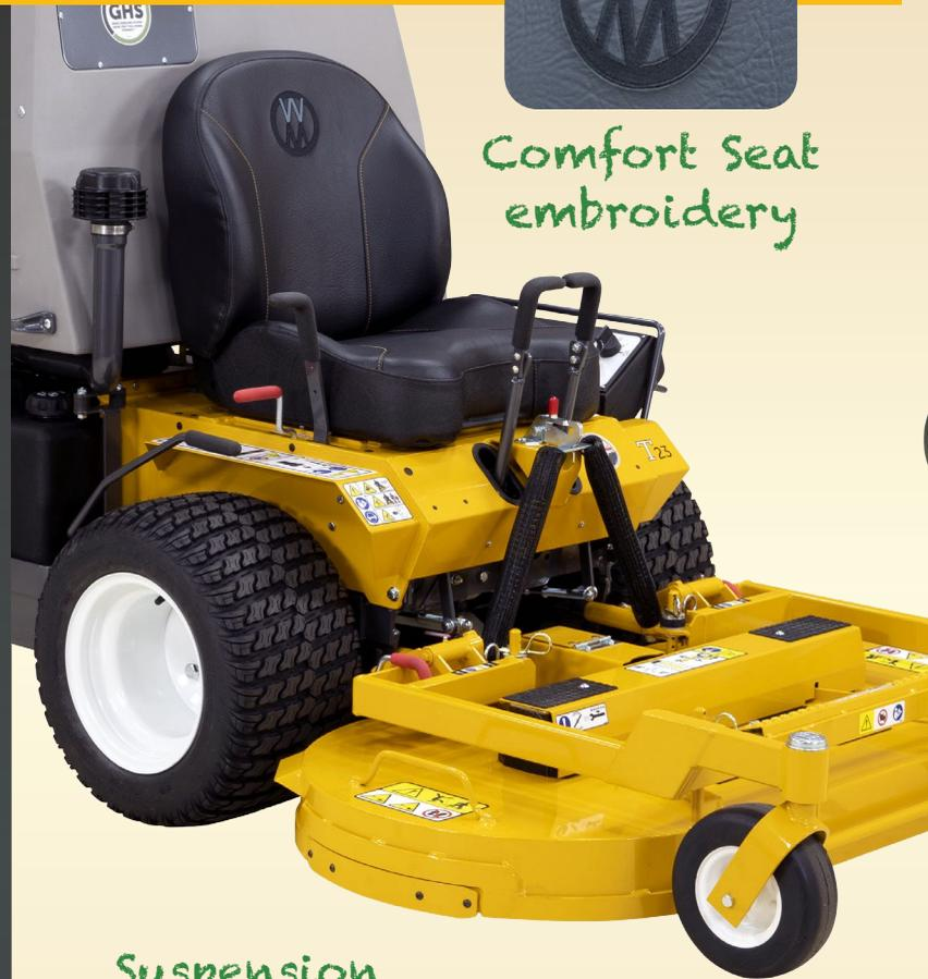
Suspension Seat absorbs bumps as the mower goes over rough terrain
