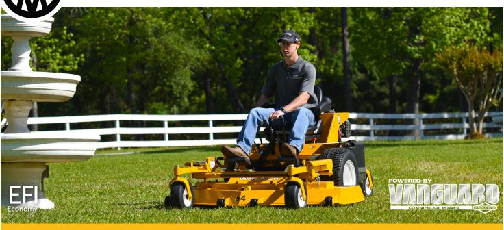
Powered by a 993cc big block Vanguard EFI engine, the H37i is a powerful and efficient machine for the professional user. Its engine debris management technology, big Donaldson air cleaner, Grammer suspension seat, and fully articulating decks means the H37i can mow complex properties easier, in harsh conditions longer. And with the optional Model H deck Power Tilt-Up, maintenance and storage are even easier.
