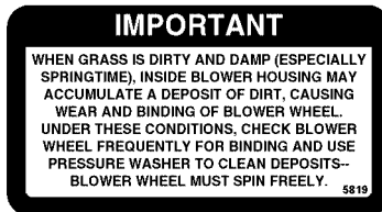
Top of Blower Housing (5819)
