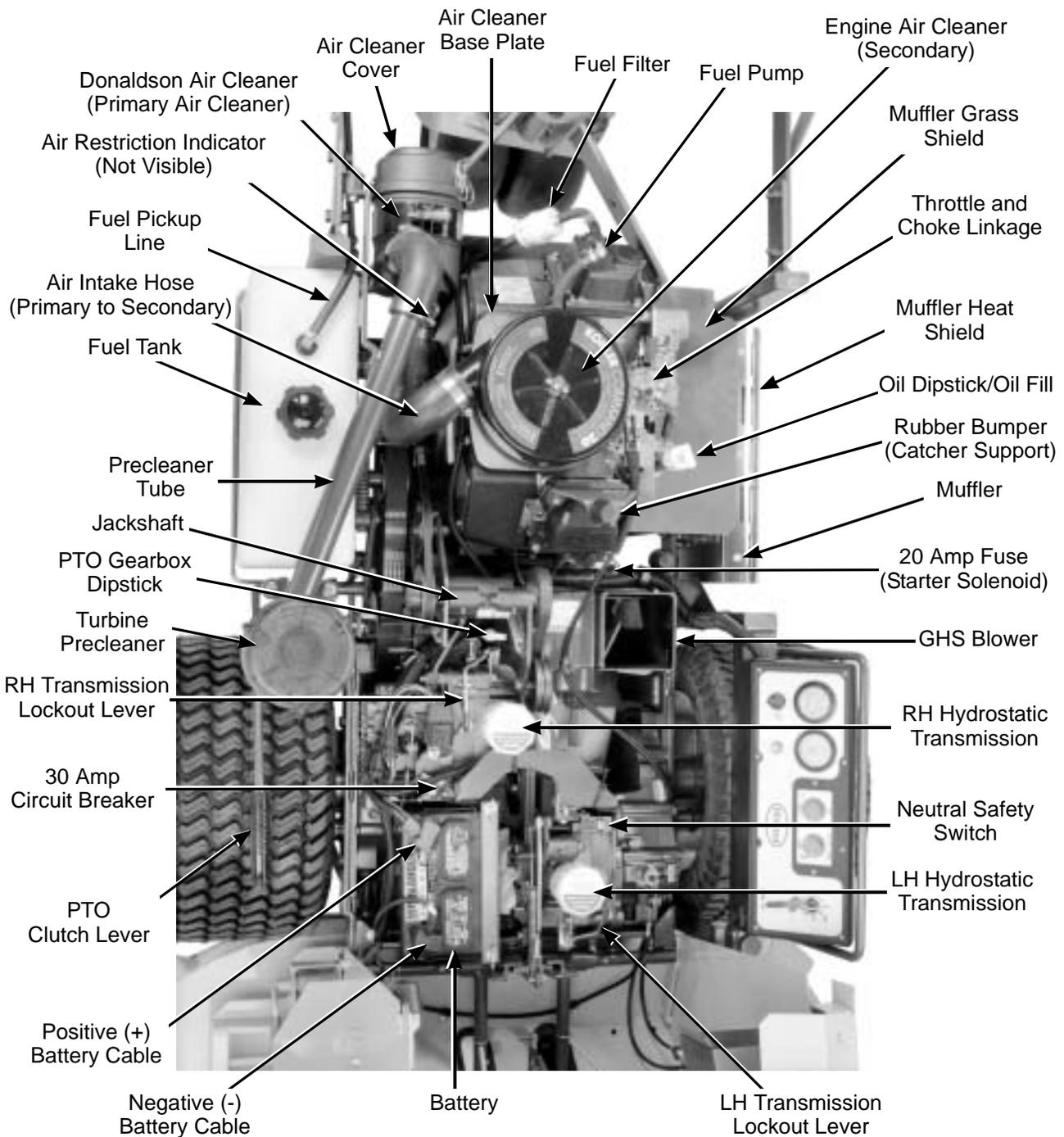
Top View (Engine Compartment) Model MT
