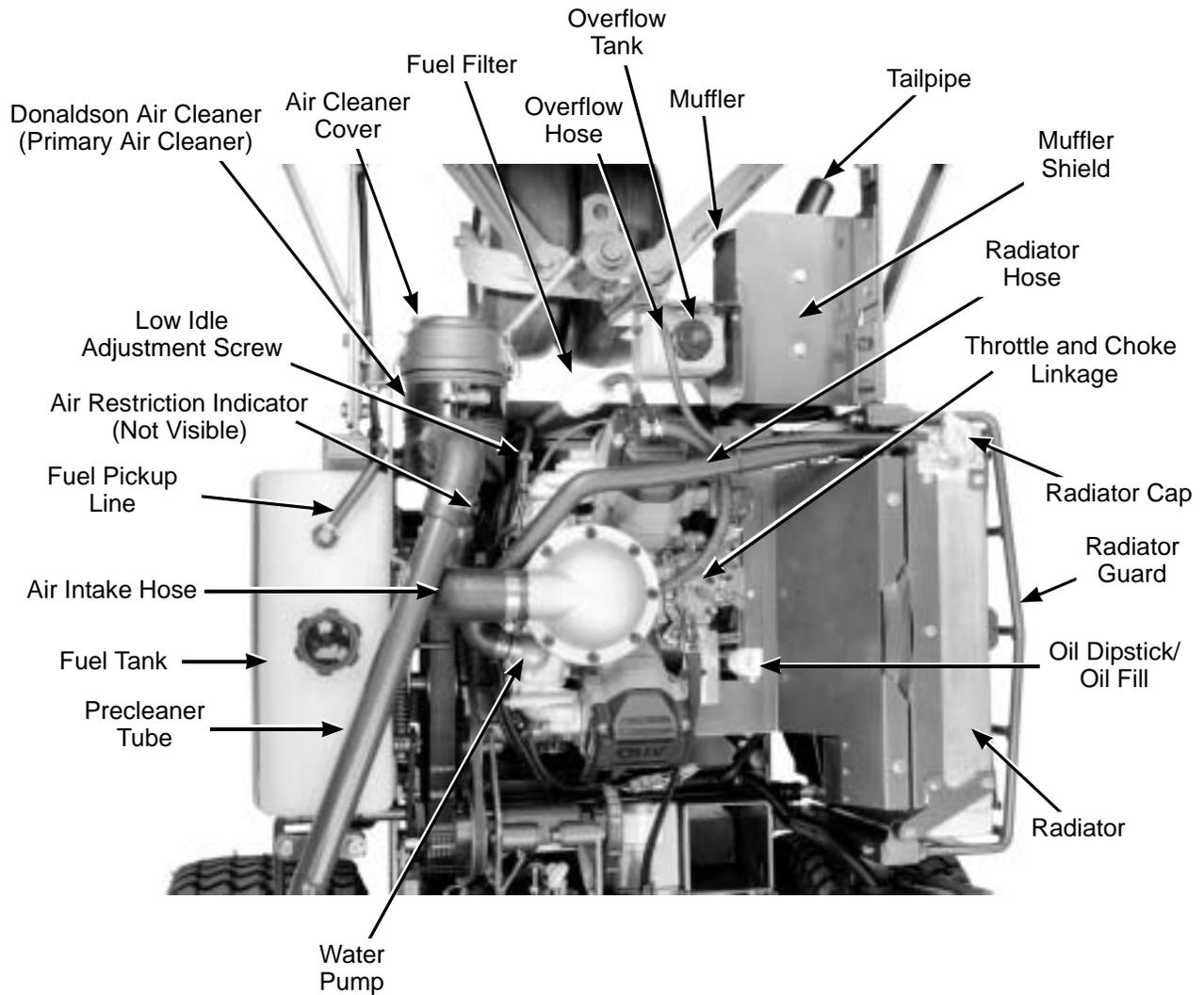
Top View (Engine Compartment) Model MTL
