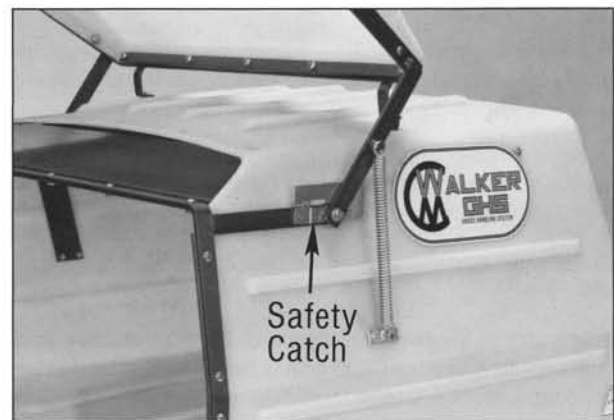
PHOTO 4-6 GHS Door Safety Catch
