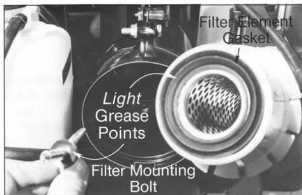
PHOTO 5-7 Air Filter Reinstallation – MD
