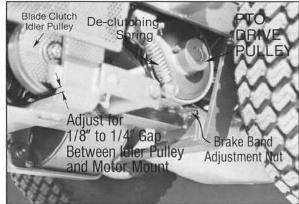
PHOTO 5-16 Blade Brake Band
