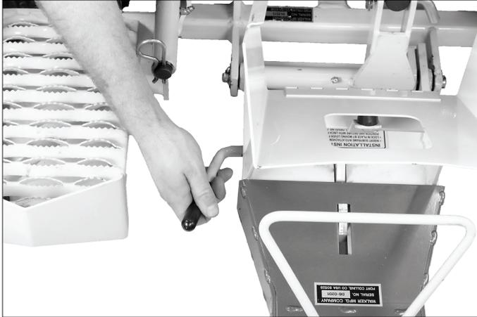
Figure 3.3 Hitch Lock Lever in "Locked" Position
