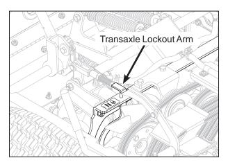
Transaxle Lockout Arm - Normal Operating Position
