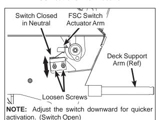
FSC Switch Adjustment (Side View Through Chassis)
