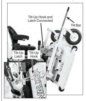
**Deck Secured in TILT-UP Position**
