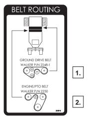
Location: Underside of Panel Behind Operator Seat
