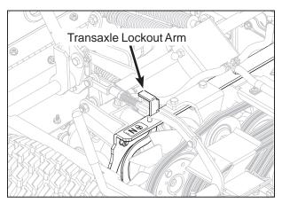
Transaxle Lockout Arm - Freewheel Position
