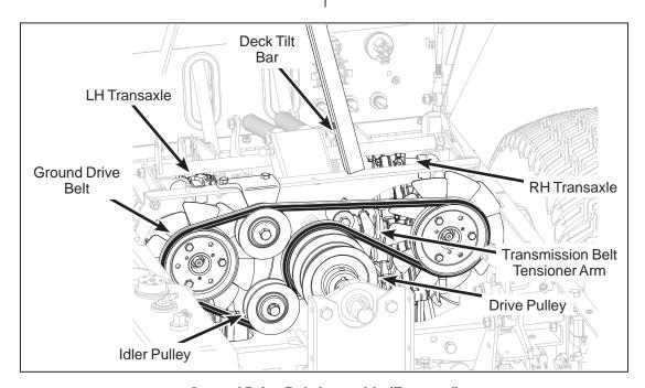
**Ground Drive Belt Assembly (Engaged)**
