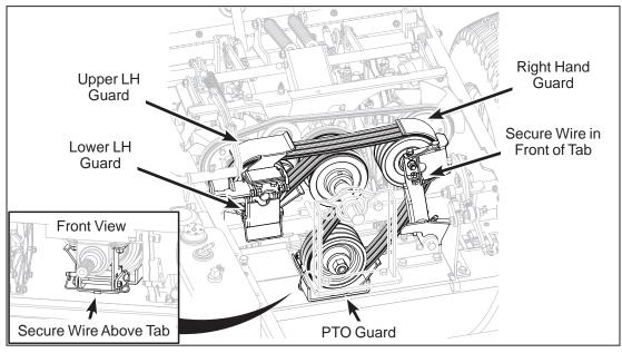
PTO Belt (Belt Guards Closed) (Engine Hidden for Clarity)
