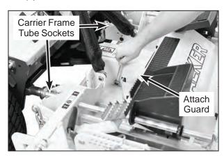
**PTO Shaft Guard Installation**
