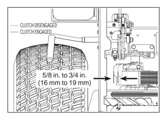
**Clutch Idler Pulley Travel Adjustment**
