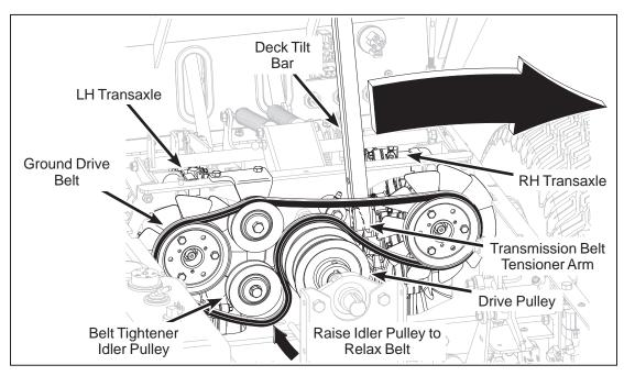
**Ground Drive Belt Assembly (Disengaged)**
