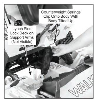
**Deck Counterweight Spring Installation**
