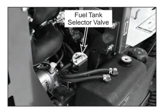
**Fuel Tank Selector Valve** (RH Side View)
