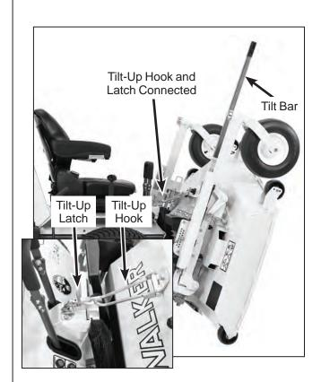
**Deck Secured in TILT-UP Position**
