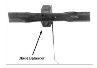
Blade Balanced on Magnetic Wall-Mounted Balancer
