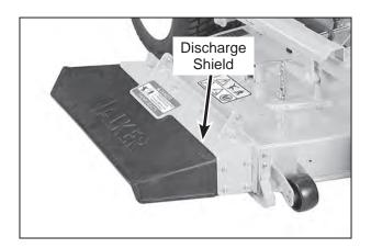
Side Discharge Deflector Shield in **Lowest Position**
