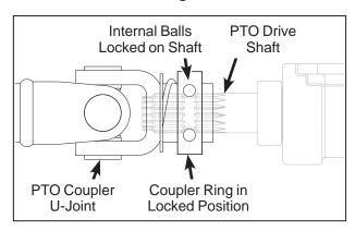
**Quick Disconnect Ring "Locked" Position**
