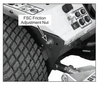
**FSC Friction Adjustment Nut**
