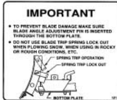
Trip Spring Lockout (RAD P/N 657503)
