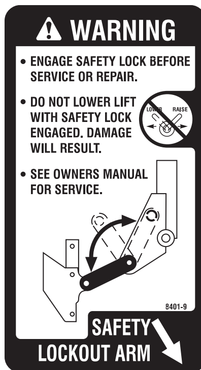
Safety Decal: Safety Lockout Arm Location: Lower Lift Arm Part Number: 8401-9
