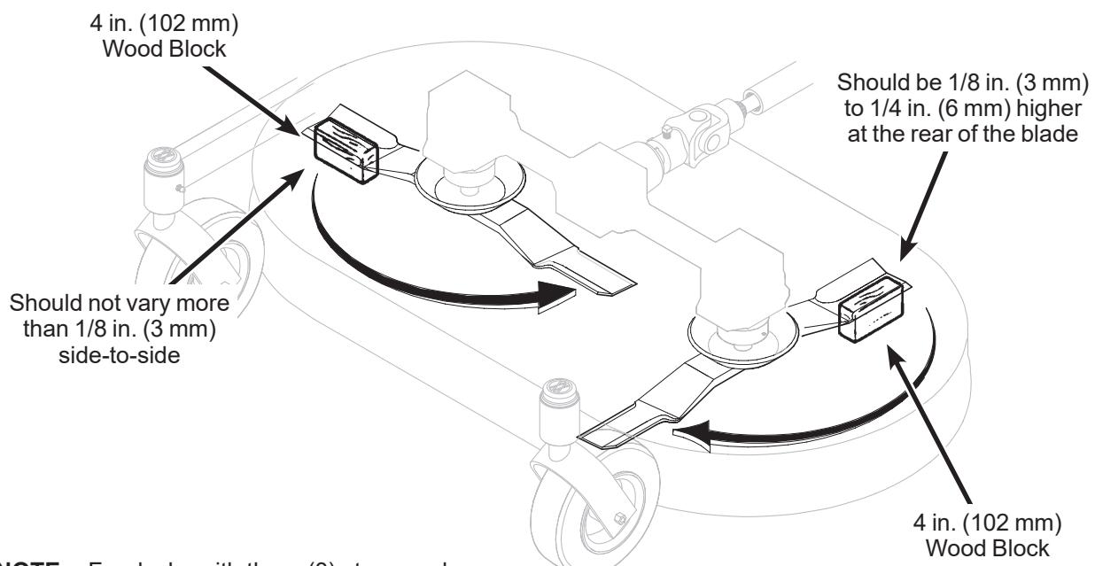
**NOTE:** For decks with three (3) staggered blades, like the DS52, the front-to-rear level should be set using the middle blade pointing forward, and either outside blade pointing back.
