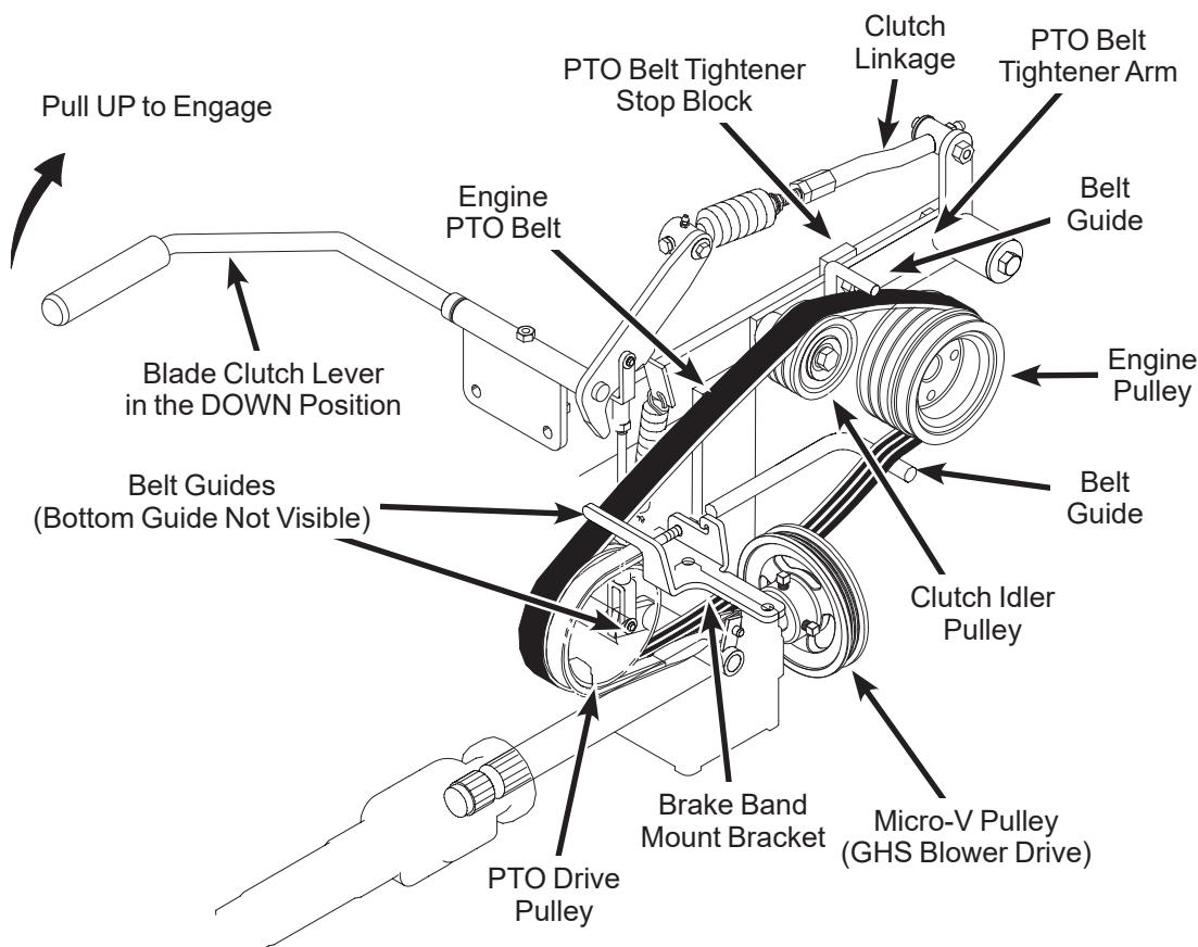
**Engine PTO Drive Belt Removal**
