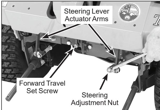
**Forward Speed Control Stop and Steering Lever Adjustment**
