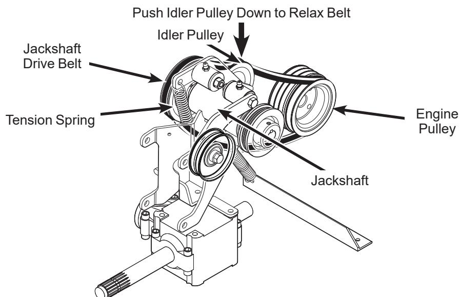
**Jackshaft Drive Belt (Disengaged)**
