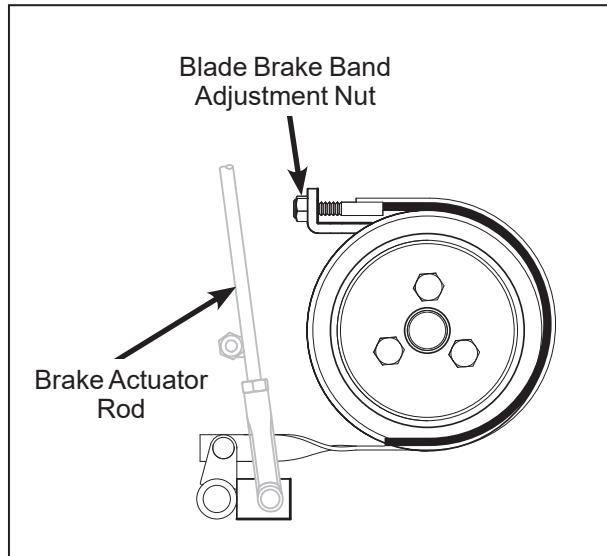
**Blade Brake Band Adjustment**
