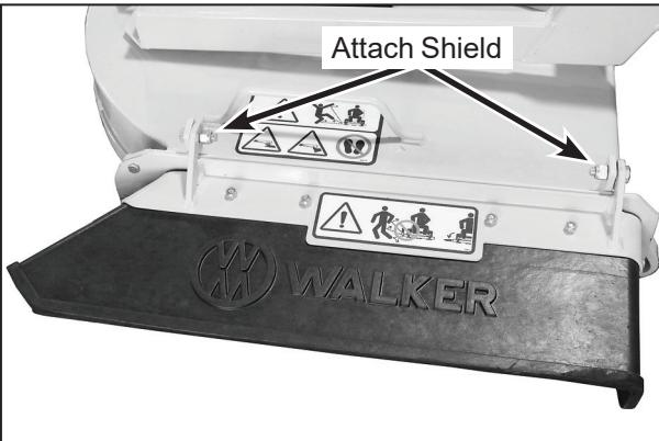
**Discharge Shield Installation
