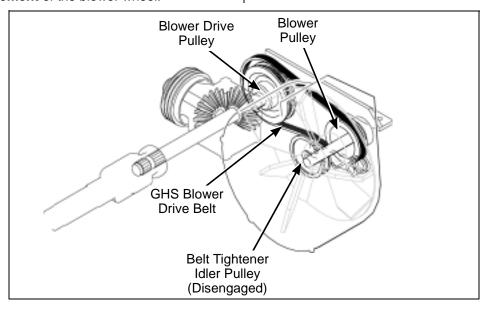
GHS Blower Drive Belt Assembly (Disengaged)
