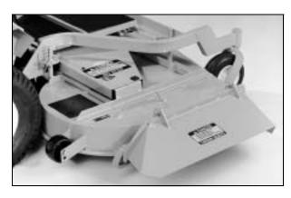
Side Discharge Shield in Lowest Position
