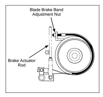
**Blade Brake Band Adjustment**
