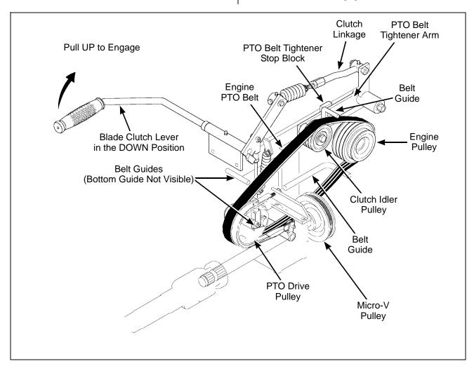
**Engine PTO Drive Belt Removal**
