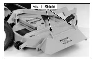
Discharge Shield Installation on Side Discharge Deck
