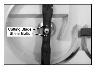
**Cutting Blade Shear Bolts**
