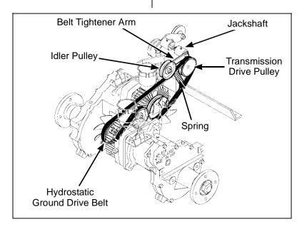
**Hydrostatic Ground Drive Belt Assembly (Disengaged)**
