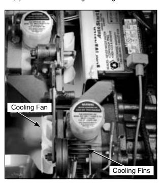
**Hydrostatic Transmission Cooling Fins**
