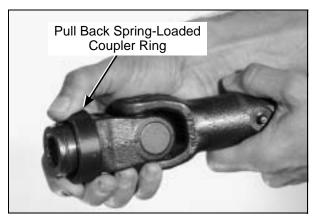
**Installing PTO Quick Coupler**
