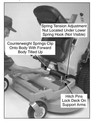
**Deck Counterweight Spring Installation**
