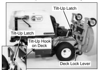
**Deck Secured in TILT-UP Position**
