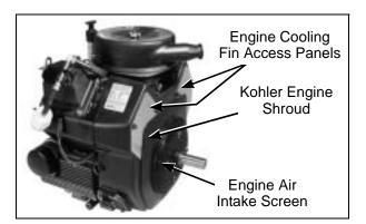
Engine Air Intake Screen and Cooling Fin Access Panels
