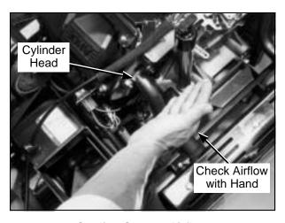
**Cooling System Airflow**
