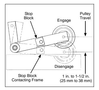
**Clutch Idler Pulley Travel Adjustment**
