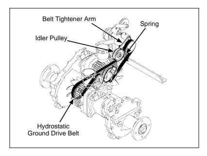
**Hydrostatic Ground Drive Belt Assembly (Engaged)**
