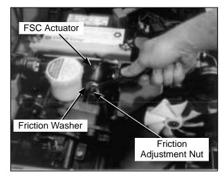
**Forward Speed Control Friction Lock**
