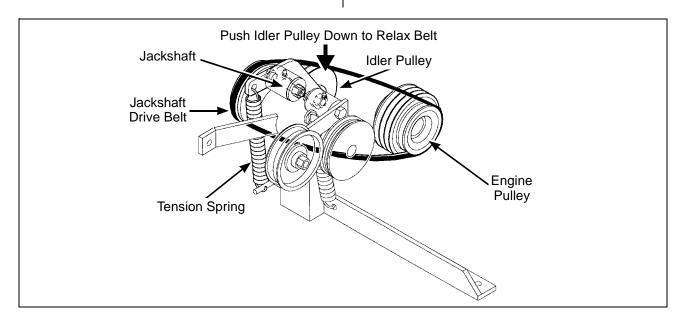
**Jackshaft Drive Belt (Disengaged)**
