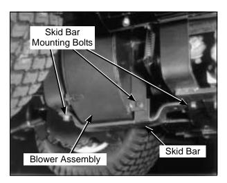
Remove Skid Bar for GHS Blower Removal
