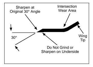
Mower Blade Profile For Sharpening
