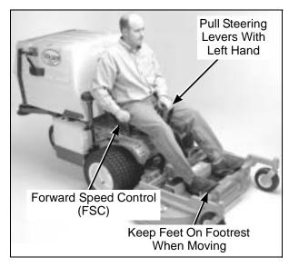
**Correct Operator Hand Position** on the Controls
