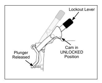
**Lockout Lever - Normal Operating Position**
