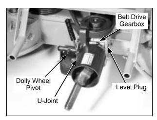
Gearbox, Dolly Wheel, and U-Joint Lubrication
