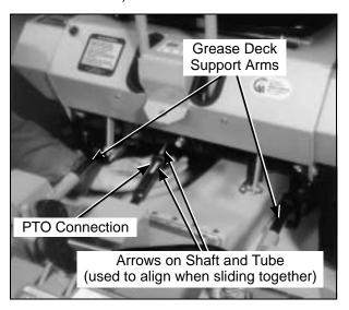
Mower Deck Installation (PTO Shaft Connection)
