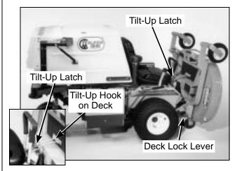
**Deck Secured in TILT-UP Position**
