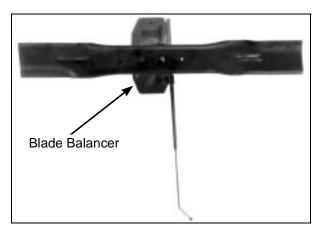
Blade Balanced on Magnetic Wall-Mounted Balancer
