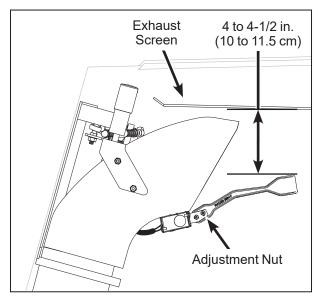
Adjusting the Grass-Pak<sup>®</sup> Switch (Side View of Catcher Box)
