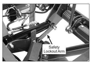
Safety Lockout Arm Engaged Position
