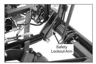
Safety Lockout Arm Disengaged Position
