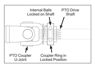
**Quick Disconnect Ring "Locked" Position**
