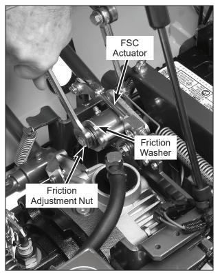
**Forward Speed Control Friction Lock**
