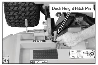
**Remove One Deck Height Hitch Pin**
