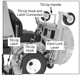
**Deck Secured in TILT-UP Position**
