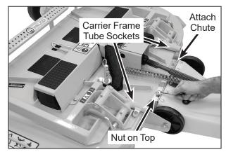
Discharge Chute Installation on Collection Deck
