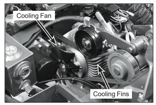
Hydrostatic Transmission Cooling Fins
