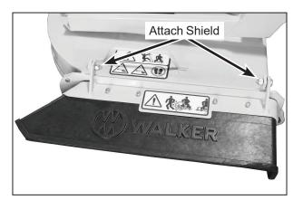
Discharge Shield Installation on Side Discharge Deck
