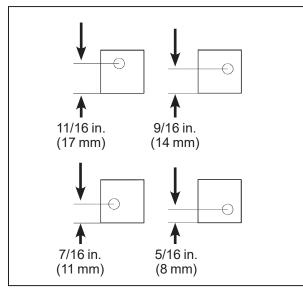
PTO Belt Tightener Stop Block Adjustments
