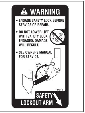
Decal, Safety Lockout Arm (Location: Lower Lift Arm)
