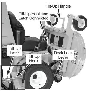
**Deck Secured in TILT-UP Position**
