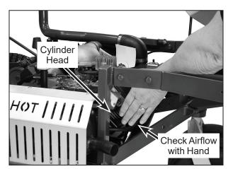
**Check Cooling System Airflow**
