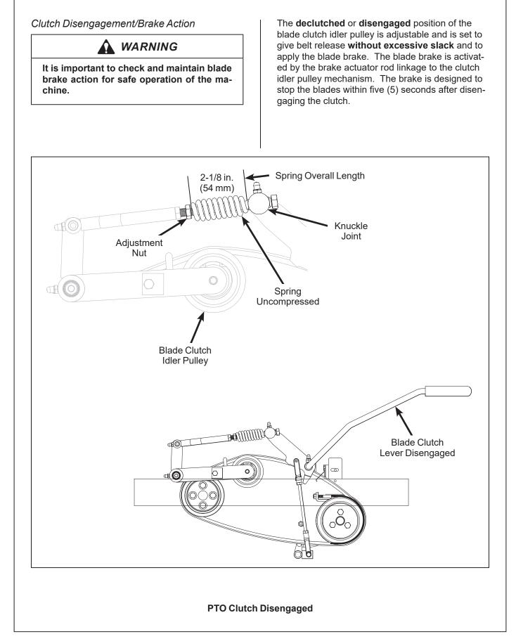
Use the following procedure to check and adjust clutch disengagement and brake action:
