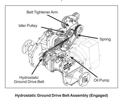
b. Slide belt off pulleys, then release the idler.
