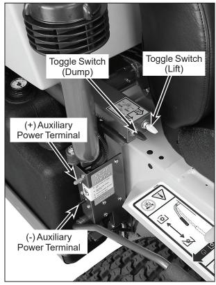
Lift/Dump Control Switches and Auxiliary Power Terminals
