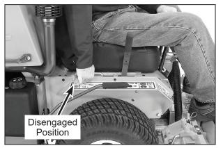
Parking Brake Disengaged
