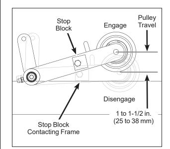
**Clutch Idler Pulley Travel Adjustment**
