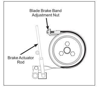
Blade Brake Band Adjustment
