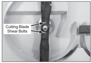
**Cutting Blade Shear Bolts**
