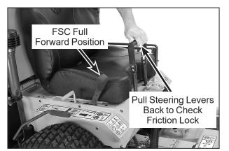
Forward Speed Control Position (Checking Friction Lock)
