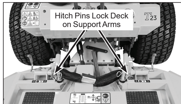
Use Hitch Pins to Lock Deck on Support Arms
