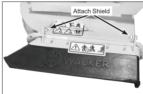
Discharge Shield Installation on Side Discharge Deck
