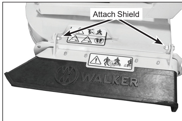
Discharge Shield Installation on Side Discharge Deck
