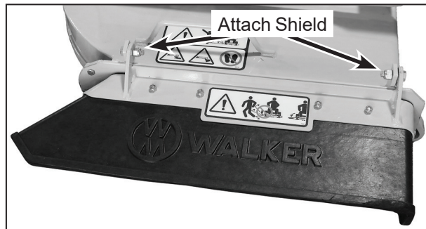
Discharge Shield Installation on Side Discharge Deck
