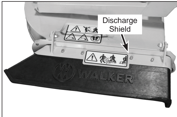
Side Discharge Deflector Shield in Lowest Position
