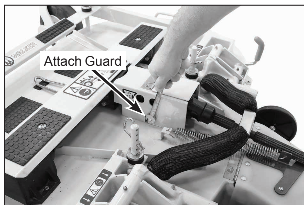
PTO Shaft Guard Installation
