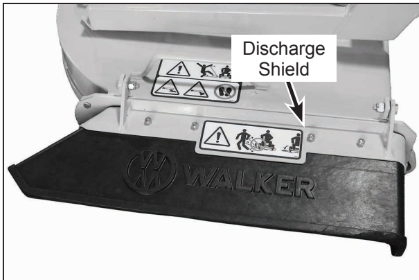
Side Discharge Deflector Shield in Lowest Position
