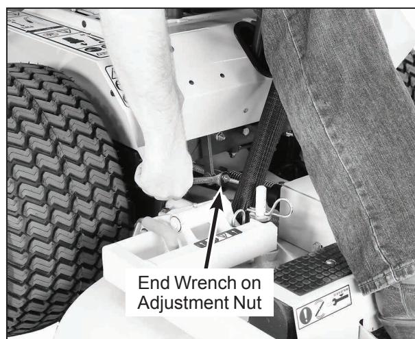
Straight Ground Travel Adjustment
