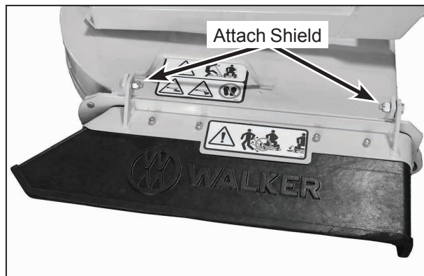
Discharge Shield Installation on Side Discharge Deck
