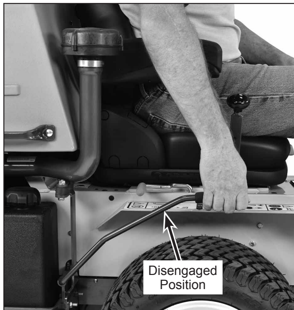
Blade Clutch Disengaged
