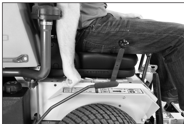
Parking Brake Disengaged
