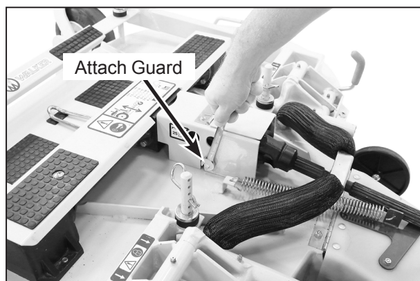
PTO Shaft Guard Installation
