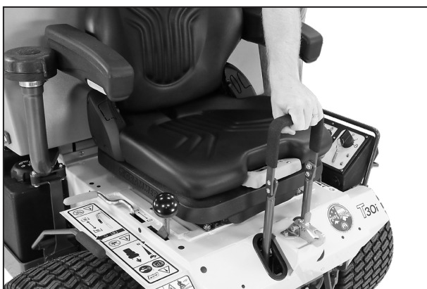
Forward Speed Control Position (Checking Friction Lock)
