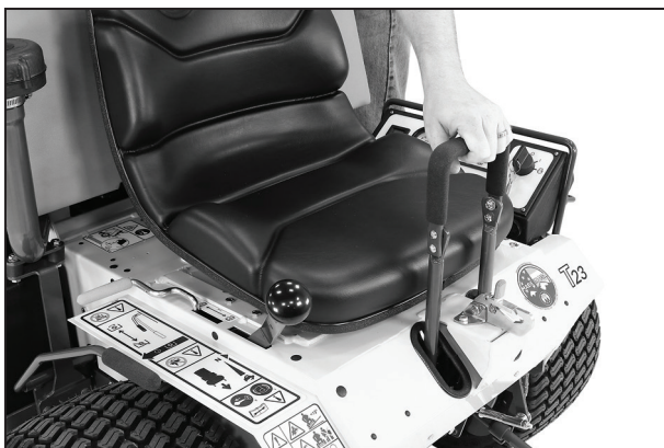
Forward Speed Control Position (Checking Friction Lock)
