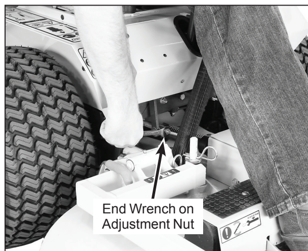
Straight Ground Travel Adjustment
