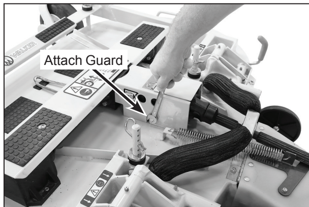
PTO Shaft Guard Installation
