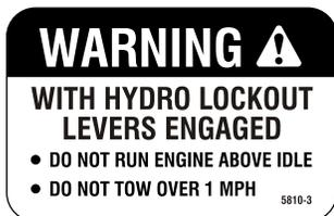
**Location: Bridge Assembly and LH Gear Axle**
