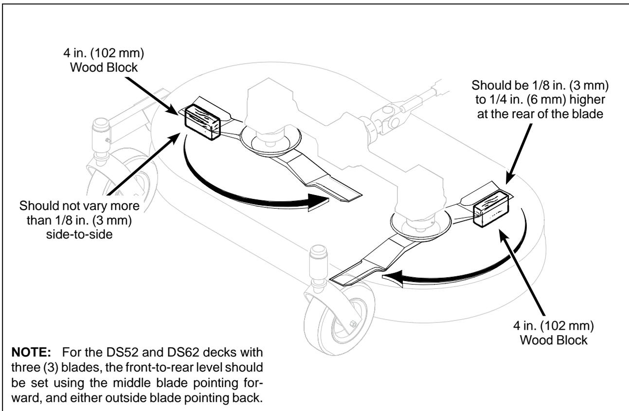
**NOTE:** For the DS52 and DS62 decks with three (3) blades, the front-to-rear level should be set using the middle blade pointing forward, and either outside blade pointing back.
