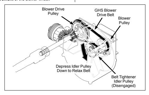
**GHS Blower Drive Belt Assembly (Disengaged)**
