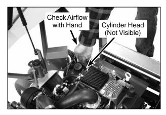
**Cooling System Airflow**
