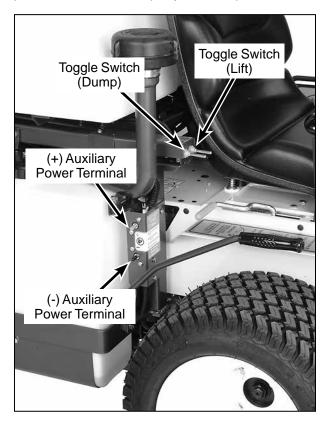
Lift/Dump Control Switches and **Auxiliary Power Terminals**
