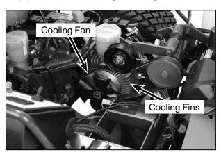
**Hydrostatic Transmission Cooling Fins**
