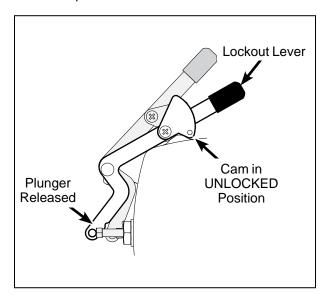
**Lockout Lever - Normal Operating Position**
