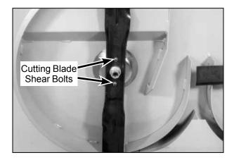
**Cutting Blade Shear Bolts**
