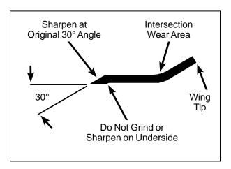
**Mower Blade Profile for Sharpening**
