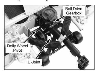
Gearbox, Dolly Wheel, and U-Joint Lubrication
