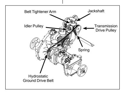
**Hydrostatic Ground Drive Belt Assembly (Disengaged)**
