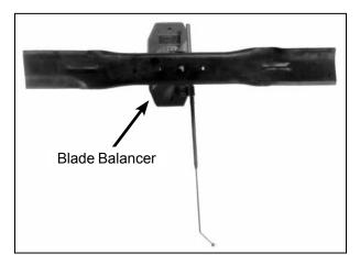
Blade Balanced on Magnetic Wall-Mounted Balancer
