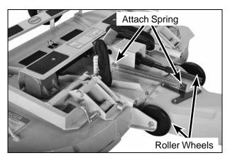
Tilt-Up Spring and Roller Wheel Installation on Rear Discharge Deck
