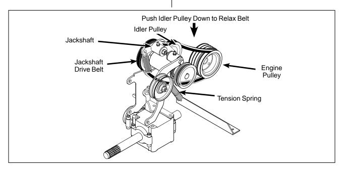
**Jackshaft Drive Belt (Disengaged)**
