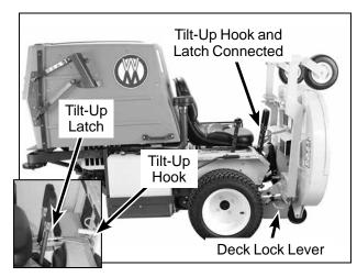
**Deck Secured in TILT-UP Position**
