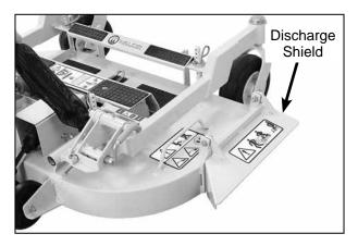
Side Discharge Deflector Shield in Lowest Position
