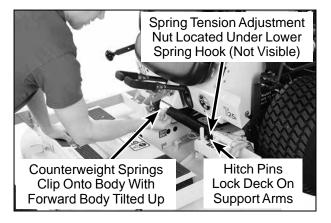
**Deck Counterweight Spring Installation**
