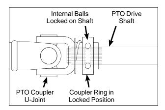
**Quick Disconnect Ring "Locked" Position**
