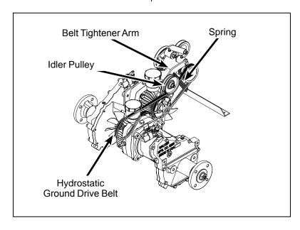
**Hydrostatic Ground Drive Belt Assembly (Engaged)**
