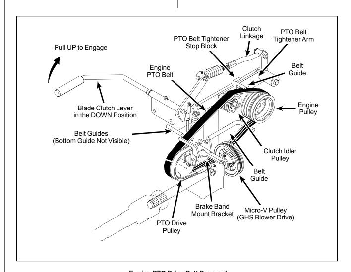
**Engine PTO Drive Belt Removal**
