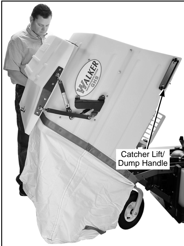
Dumping Catcher into Dump Bag
