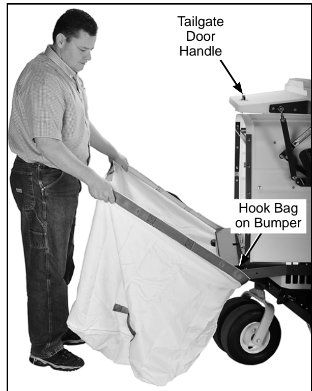
Positioning Dump Bag on Catcher
