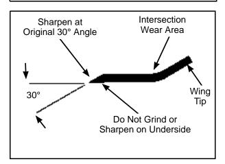
Mower Blade Profile For Sharpening
