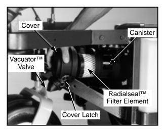
Air Cleaner Components (shown with cover being removed)
