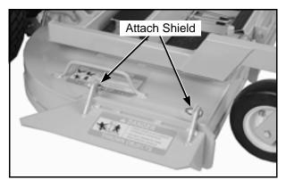
Discharge Shield Installation on Side Discharge Deck
