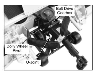
Gearbox, Dolly Wheel, and U-Joint Lubrication
