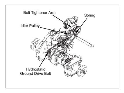
**Hydrostatic Ground Drive Belt Assembly (Engaged)**
