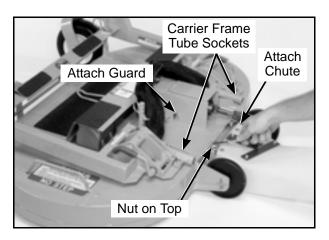
Discharge Chute and PTO Shaft Guard Installation on Rear Discharge Deck
