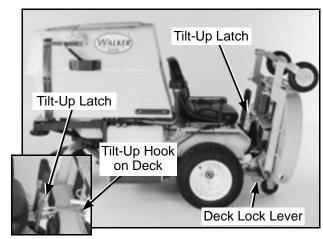
**Deck Secured in TILT-UP Position**
