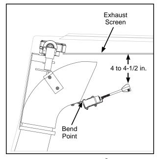
Adjusting the Grass-Pak<sup>®</sup> Switch (Side view of Catcher Box)
