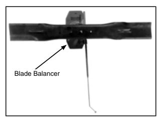
Blade Balanced on Magnetic Wall-Mounted Balancer
