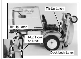
**Deck Secured in TILT-UP Position**
