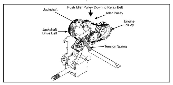
**Jackshaft Drive Belt (Disengaged)**
