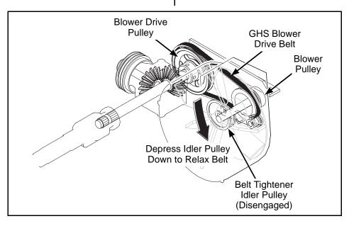
GHS Blower Drive Belt Assembly (Disengaged)
