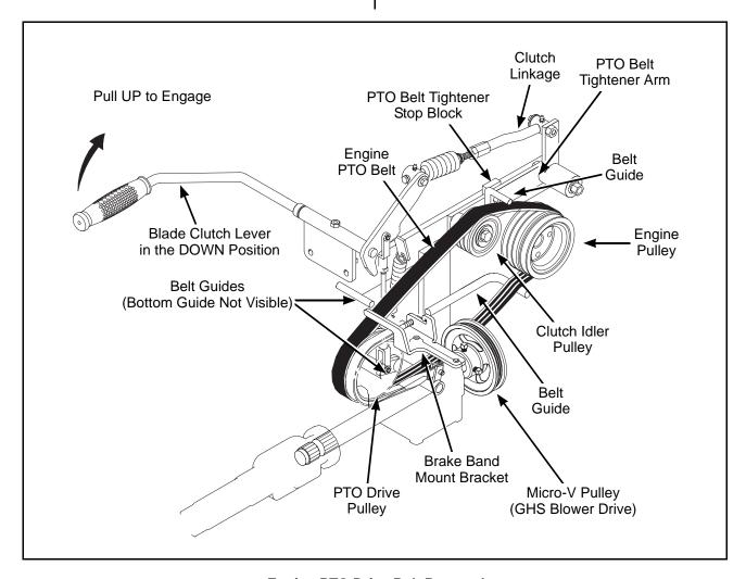
**Engine PTO Drive Belt Removal**
