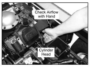
**Cooling System Airflow**
