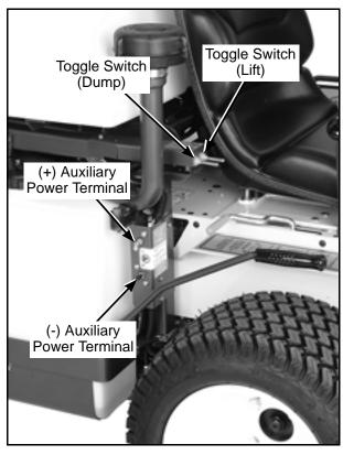
Lift/Dump Control Switches and Auxiliary Power Terminals
