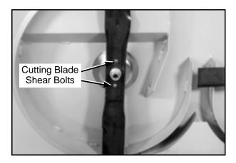
**Cutting Blade Shear Bolts**
