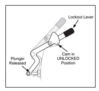
**Lockout Lever - Normal Operating Position**
