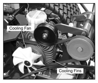
**Hydrostatic Transmission Cooling Fins**
