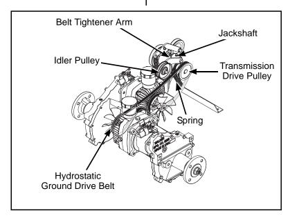
**Hydrostatic Ground Drive Belt Assembly (Disengaged)**
