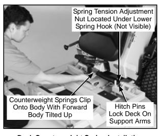
**Deck Counterweight Spring Installation**
