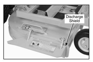
**Side Discharge Shield in Lowest Position**
