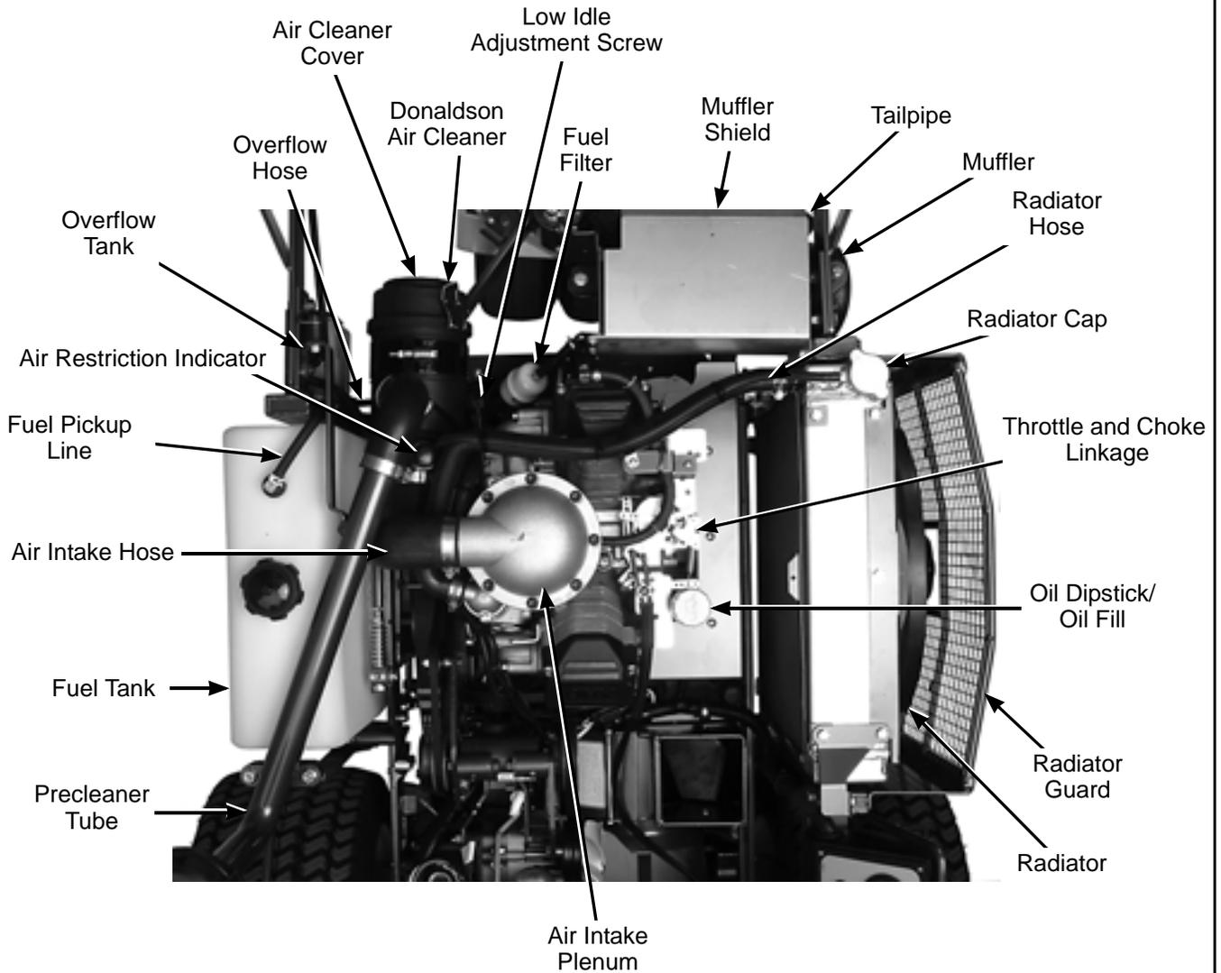
Top View (Engine Compartment) Model MTL
