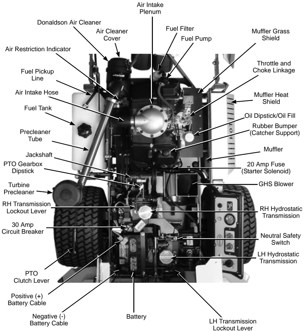
Top View (Engine Compartment) Model MT
