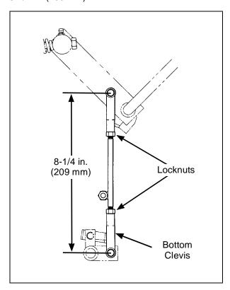
**Brake Actuator Rod Adjustment**
