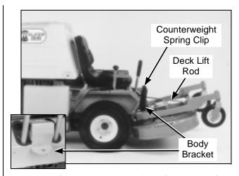
**Deck Secured in UP Position (Non-Tilting)**
