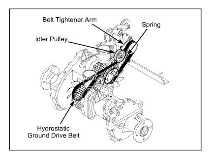
**Hydrostatic Ground Drive Belt Assembly (Engaged)**
