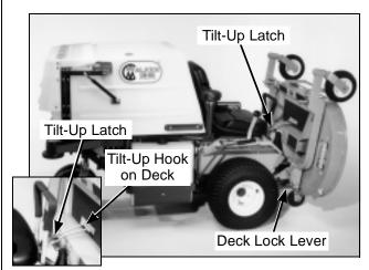
**Deck Secured in TILT-UP Position**
