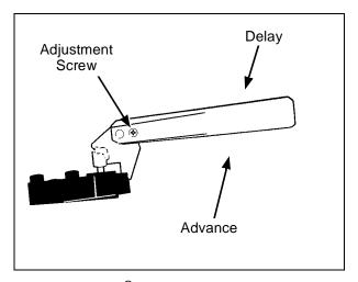
Grass-Pak® Switch Vane Adjustment
