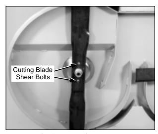
**Cutting Blade Shear Bolts**
