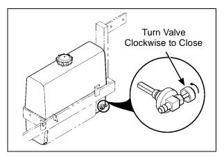
**Fuel Shut-Off Valve and Filter**
