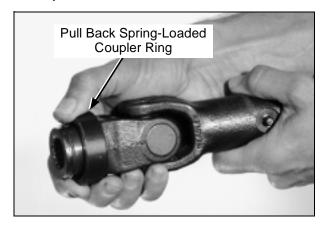
**Installing PTO Quick Coupler**
