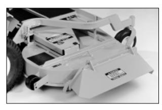
**Side Discharge Shield in Lowest Position**
