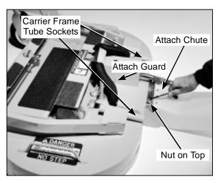
Discharge Chute and PTO Shaft Guard Installation on Rear Discharge Deck
