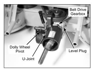
Gearbox, Dolly Wheel, and U-Joint Lubrication
