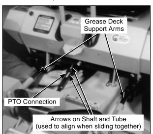
Mower Deck Installation (PTO Shaft Connection)
