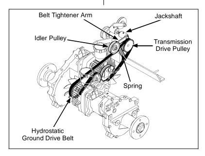
**Hydrostatic Ground Drive Belt Assembly (Disengaged)**
