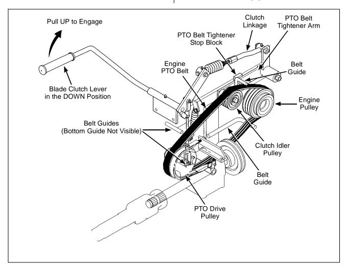
**Engine PTO Drive Belt Removal**
