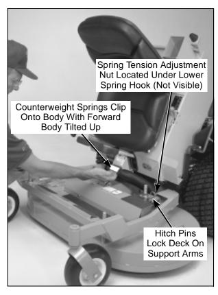
**Deck Counterweight Spring Installation**
