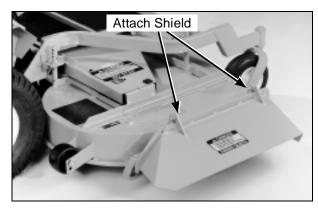
Discharge Shield Installation on Side Discharge Deck
