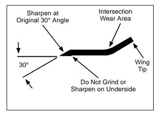
Mower Blade Profile For Sharpening
