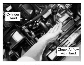
**Cooling System Airflow**
