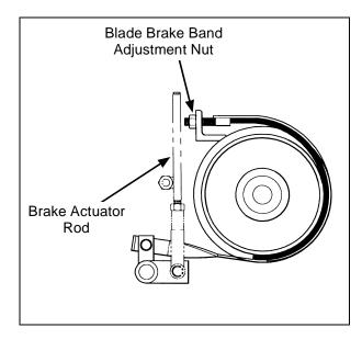
**Blade Brake Band Adjustment**
