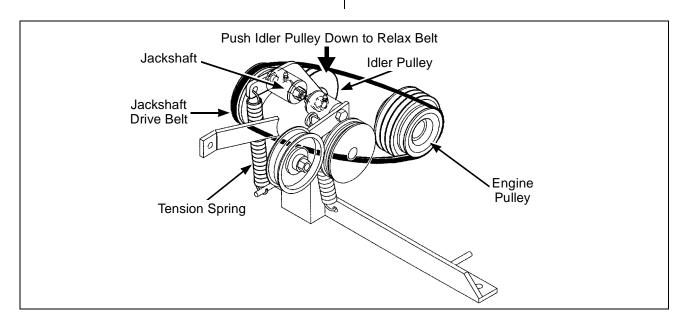
**Jackshaft Drive Belt (Disengaged)**
