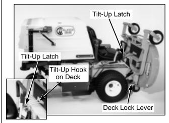
**Deck Secured in TILT-UP Position**
