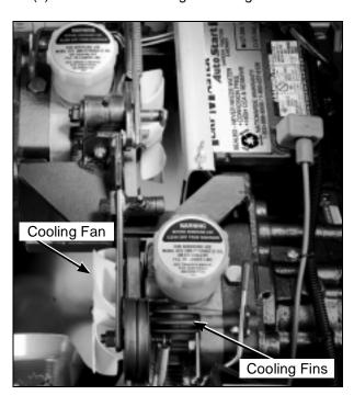
**Hydrostatic Transmission Cooling Fins**
