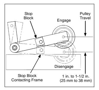
**Clutch Idler Pulley Travel Adjustment**
