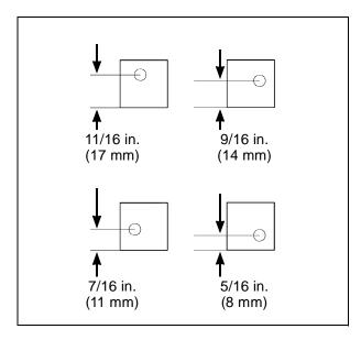
**PTO Belt Tightener Stop Block Adjustments**
