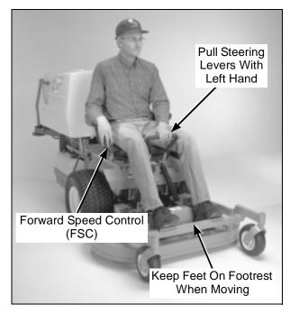
**Correct Operator Hand Position** on the Controls
