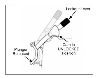
**Lockout Lever - Normal Operating Position**
