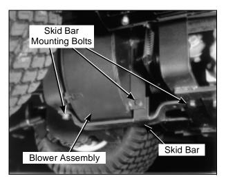
Remove Skid Bar for GHS Blower Removal
