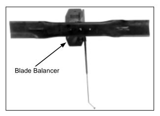
Blade Balanced on Magnetic Wall-Mounted Balancer
