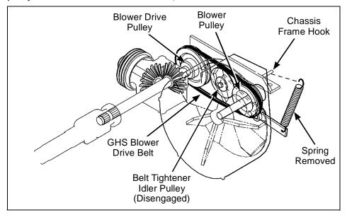
GHS Blower Drive Belt Assembly (Disengaged)
