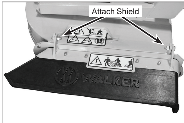
Discharge Shield Installation on Side Discharge Deck
