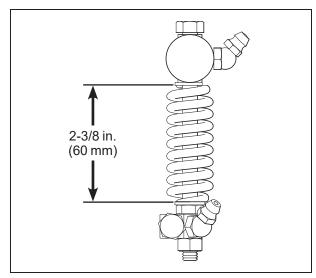
**Clutch Linkage Adjustment - Disengaged**
