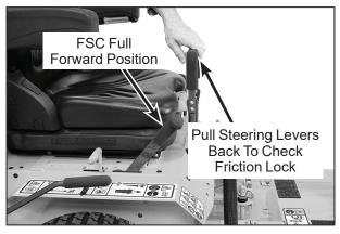
Forward Speed Control Position (Checking Friction Lock)
