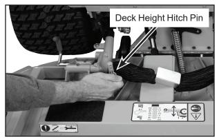
**Remove One Deck Height Hitch Pin**
