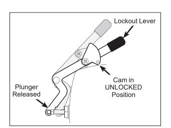
Lockout Lever - Normal Operating Position
