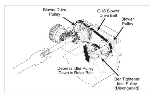
GHS Blower Drive Belt Assembly (Disengaged)
