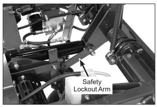
Safety Lockout Arm Engaged Position
