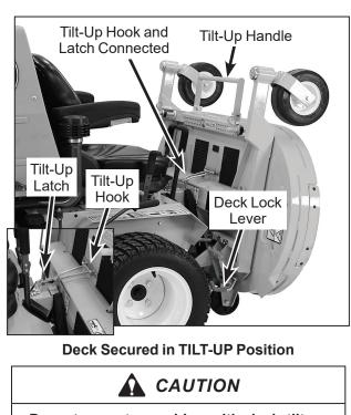
Do not operate machine with deck tilt-up pivot joint unlocked.
