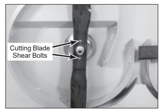
**Cutting Blade Shear Bolts**
