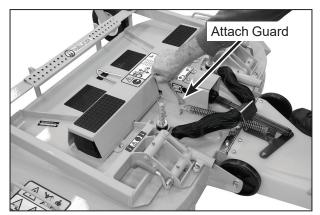
**PTO Shaft Guard Installation**
