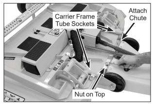
Discharge Chute Installation on Collection Deck
