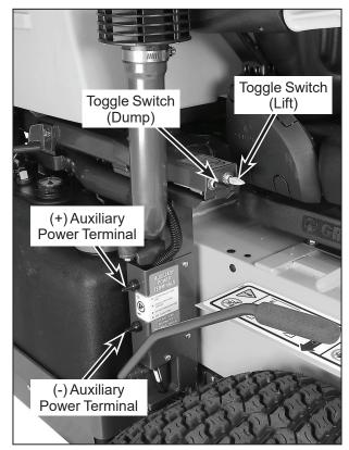
Lift/Dump Control Switches and Auxiliary Power Terminals
