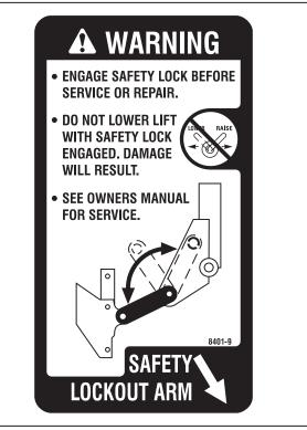
Decal, Safety Lockout Arm (Location: Lower Lift Arm)
