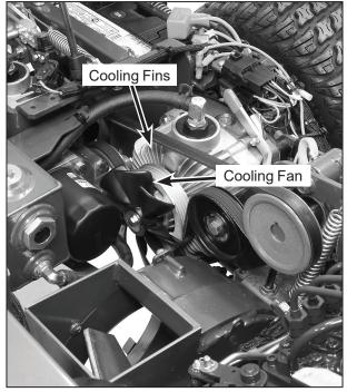
Hydrostatic Transmission Cooling Fins
