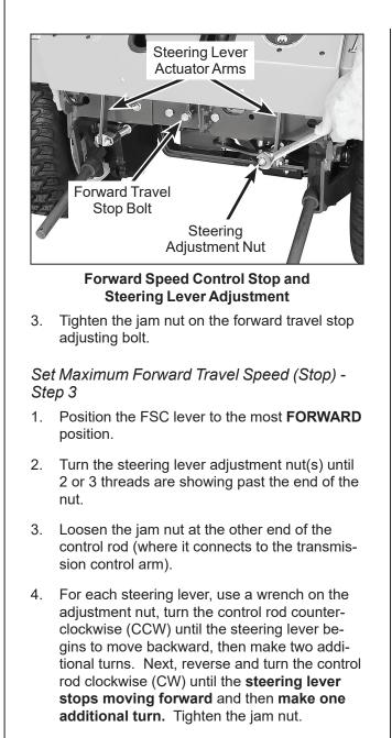
**NOTE:** Failure to make at **least one extra turn** on the control rod can place excessive loads on the transmission internal control stops and cause internal wear and damage to the transmission. Making additional turns beyond one turn reduces the maximum forward travel speed.
