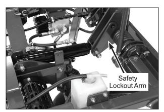
Safety Lockout Arm Disengaged Position
