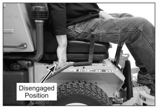
Parking Brake Disengaged
