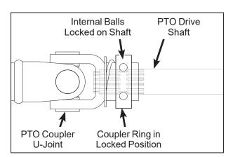
**Quick Disconnect Ring "Locked" Position**
