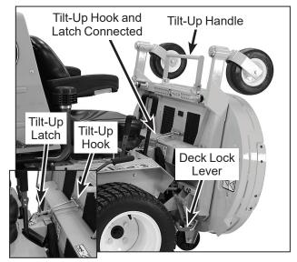
**Deck Secured in TILT-UP Position**
