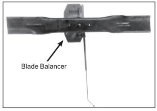
Blade Balanced on Magnetic Wall-Mounted Balancer
