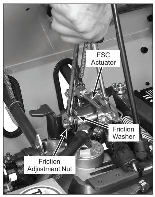
Forward Speed Control Friction Lock
