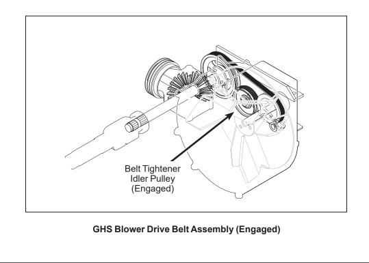
b. Slide belt off pulleys, then release the idler.
