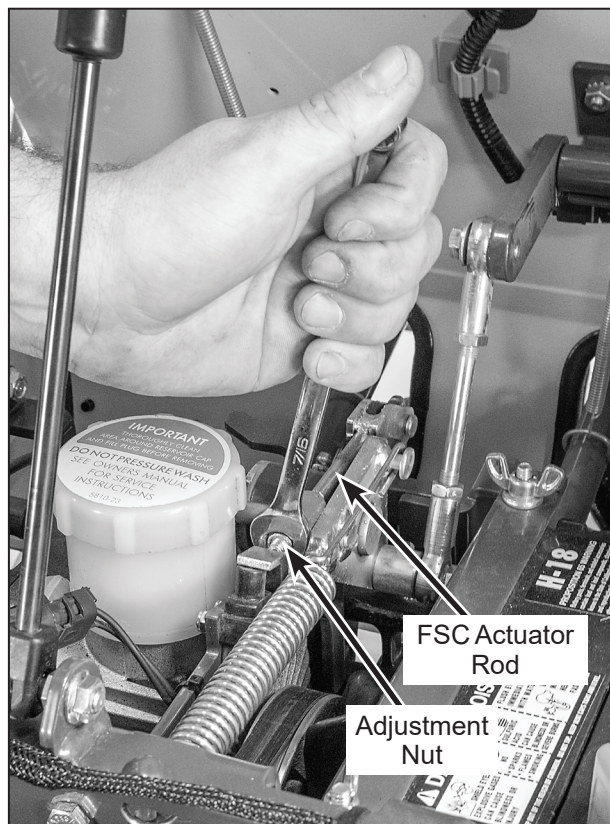
Neutral Function Adjustment
