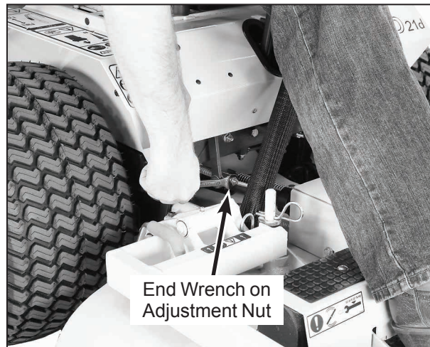
Straight Ground Travel Adjustment
