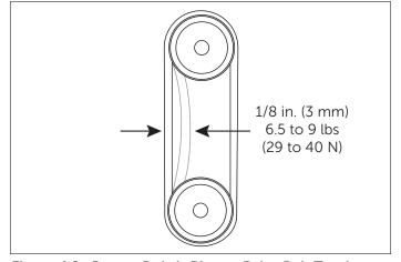
Figure 4.2: Proper Debris Blower Drive Belt Tension
