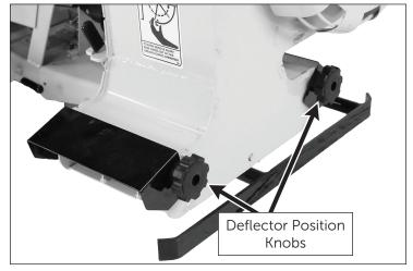
Figure 3.1: Deflector Position Knobs
