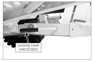
Figure 2.6: Hitch Lock Lever in "UNLOCKED" Position (View From Right Side of Tractor)
