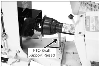
Figure 2.7: PTO Shaft Support Raised
