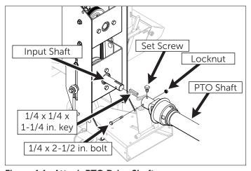
Figure 1.1: Attach PTO Drive Shaft
