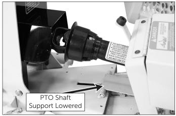
Figure 2.8: PTO Shaft Support Lowered
