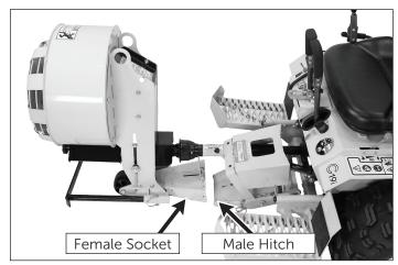
Figure 2.3: Male to Female Hitch Connection
