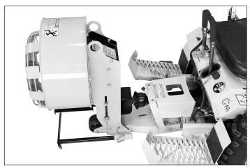
Figure 2.4: Hitch Connected to Debris Blower (View from LH Side of Tractor)
