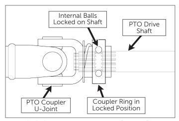
Figure 2.10: Quick Disconnect Ring in "Locked" Position
