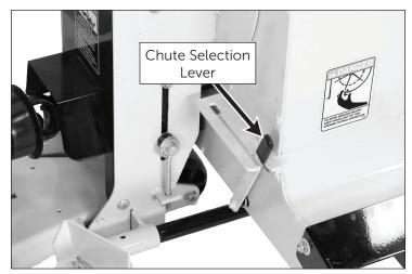
Figure 3.2: Chute Selection Lever
