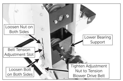
Figure 4.3: Adjusting Belt Tension
