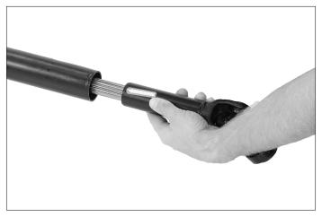
Figure 2.1: Install PTO Coupler on Drive Shaft
