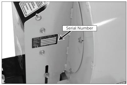
Debris Blower Serial Number Location (Rear View and RH View)
