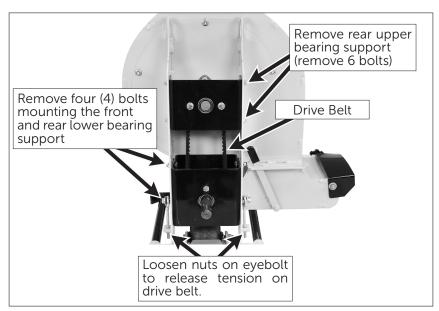
Figure 4.1: Remove Debris Blower Drive Belt
