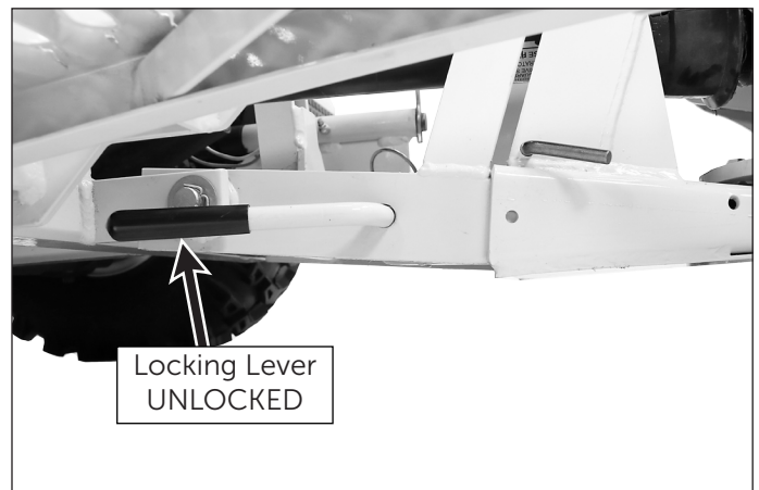
Figure 2.6: Hitch Lock Lever in "UNLOCKED" Position (View From Right Side of Tractor)
