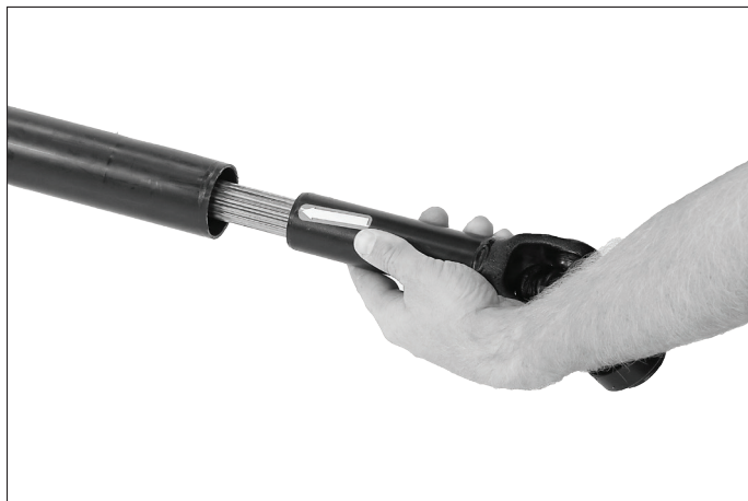
Figure 2.1: Install PTO Coupler on Drive Shaft
