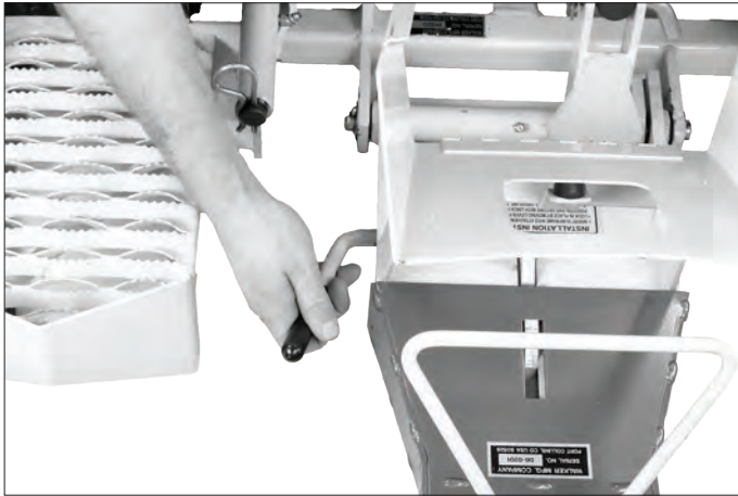
Figure 3.3 Hitch Lock Lever in "Locked" Position
