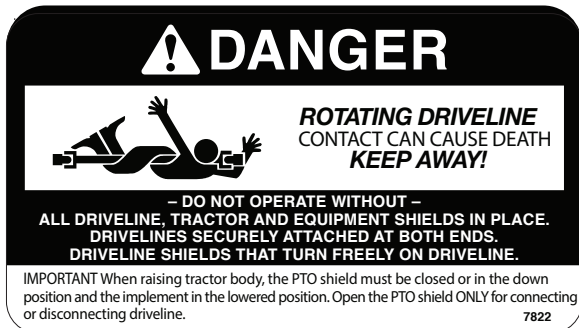
Safety Decal: Rotating Driveline Location: PTO Shield Part Number: 7822
