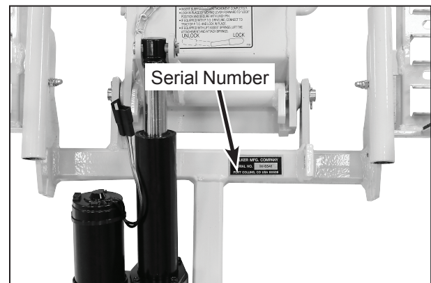
H10/H21 Implement Hitch Serial Number Location (H10 Shown, Top View)
