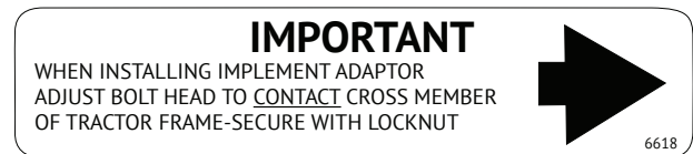
Adjustment Decal: 3/4 in. Bolt - H10 ONLY Location: Frame, H10 Implement Hitch Part Number: 6618
