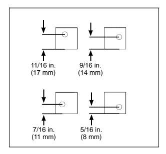
**PTO Belt Tightener Stop Block Adjustments**
