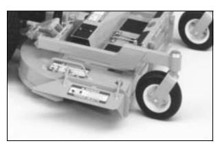
**Side Discharge Shield in Lowest Position**
