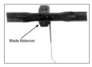
Blade Balanced on Magnetic Wall-Mounted Balancer
