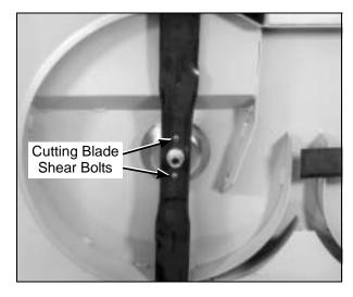
**Cutting Blade Shear Bolts**
