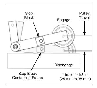
**Clutch Idler Pulley Travel Adjustment**
