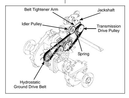
**Hydrostatic Ground Drive Belt Assembly (Disengaged)**
