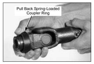
**Installing PTO Quick Coupler**
