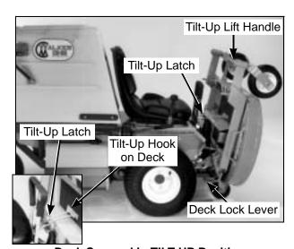
**Deck Secured in TILT-UP Position**
