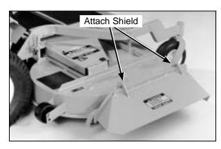
Discharge Shield Installation on Side Discharge Deck
