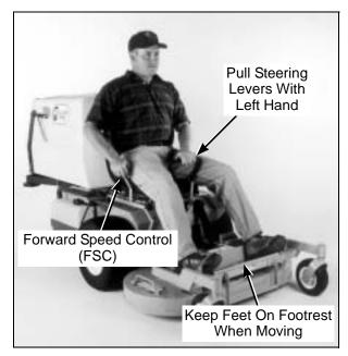
**Correct Operator Hand Position** on the Controls
