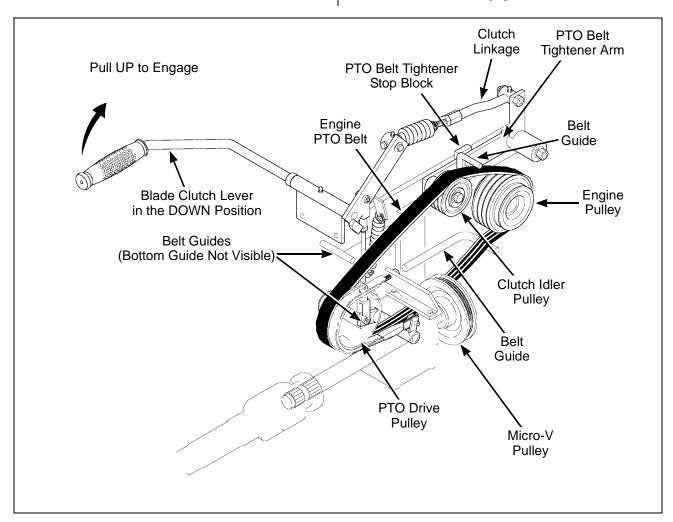
**Engine PTO Drive Belt Removal**
