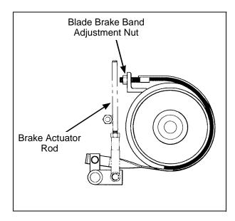
**Blade Brake Band Adjustment**
