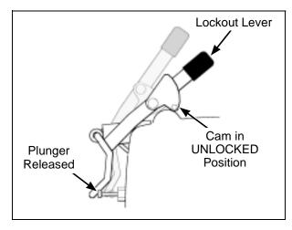
**Lockout Lever - Normal Operating Position**
