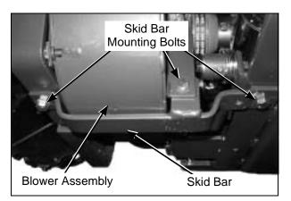
Remove Skid Bar for GHS Blower Removal
