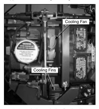
**Hydrostatic Transmission Cooling Fins**
