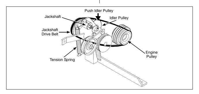
**Jackshaft Drive Belt (Disengaged)**
