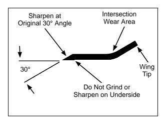
Mower Blade Profile For Sharpening
