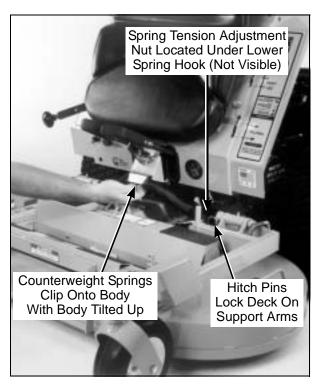
**Deck Counterweight Spring Installation**
