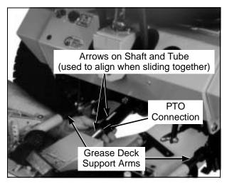
Mower Deck Installation (PTO Shaft Connection)
