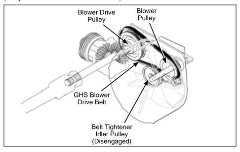
GHS Blower Drive Belt Assembly (Disengaged)
