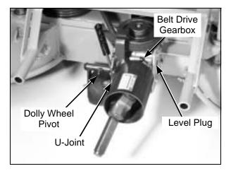
Gearbox, Dolly Wheel, and U-Joint Lubrication
