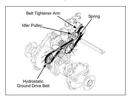
**Hydrostatic Ground Drive Belt Assembly (Engaged)**
