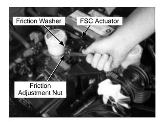
**Forward Speed Control Friction Lock**
