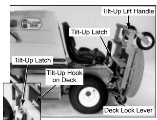
**Deck Secured in TILT-UP Position**
