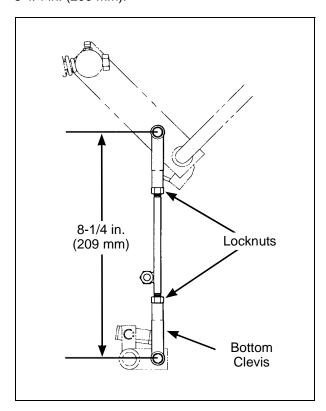
**Brake Actuator Rod Adjustment**
