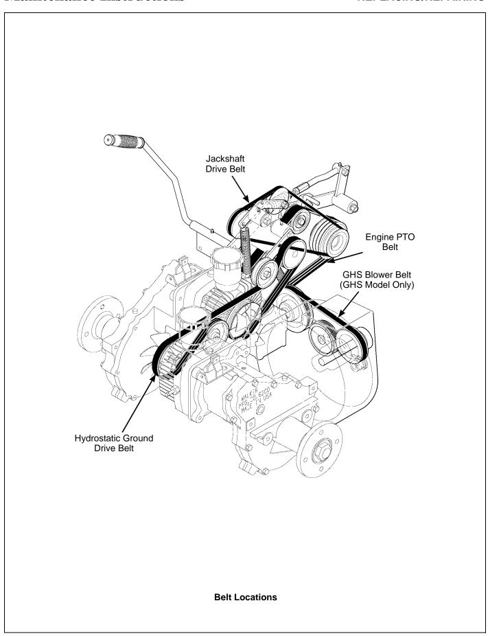
Engine PTO Drive Belt (3 Groove Power Band)
