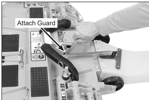
PTO Shaft Guard Installation
