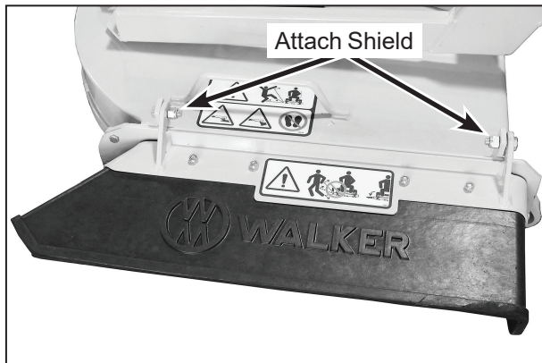
Discharge Shield Installation on Side Discharge Deck
