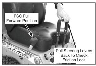
FSC Friction Adjustment Test (Checking Friction Lock)
