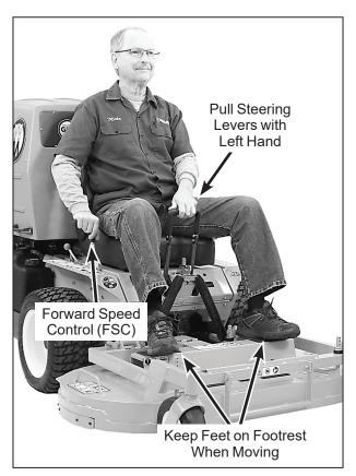
**Correct Operator Hand Position** on the Controls
