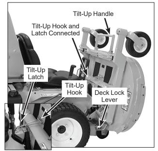
Deck Secured in TILT-UP Position
