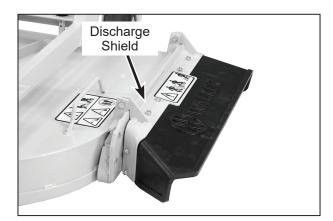
Side Discharge Deflector Shield in Lowest Position
