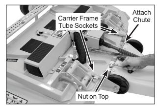
Discharge Chute Installation on Collection Deck
