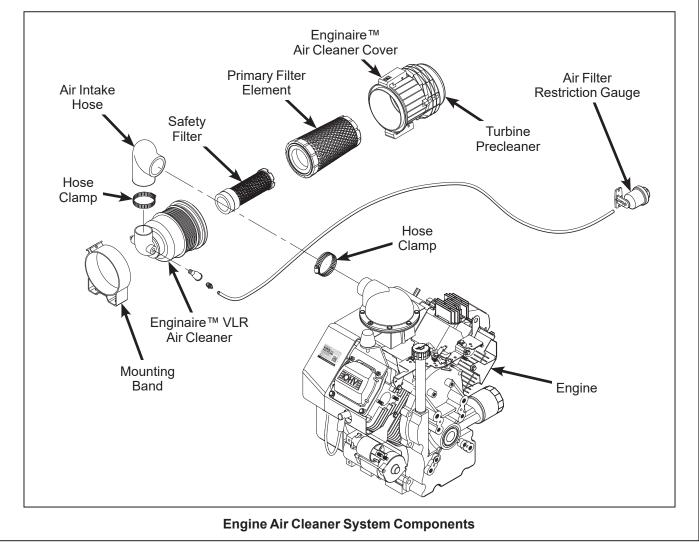
**IMPORTANT:** Use **only** Enginaire<sup>™</sup> air filter elements for replacement (Walker P/N 5090-5 and 5090-6). Aftermarket filters may not seal properly or filter efficiently.
