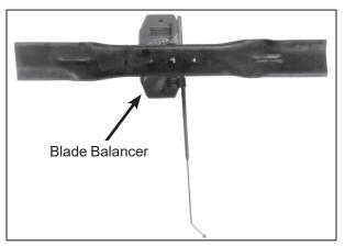
Blade Balanced on Magnetic Wall-Mounted Balancer
