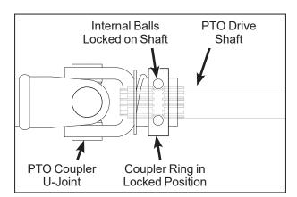
**Quick Disconnect Ring "Locked" Position**
