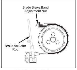
Blade Brake Band Adjustment
