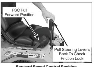
Forward Speed Control Position (Checking Friction Lock)
