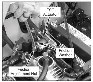
**Forward Speed Control Friction Lock**
