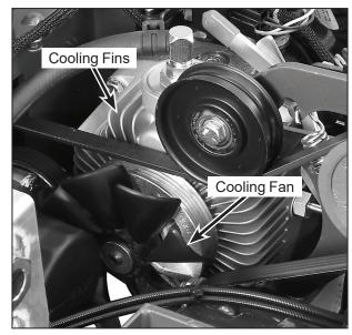
Hydrostatic Transmission Cooling Fins
