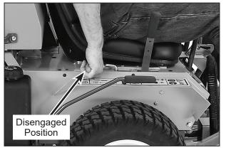
Parking Brake Disengaged
