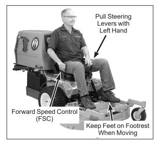
Correct Operator Hand Position on the Controls
