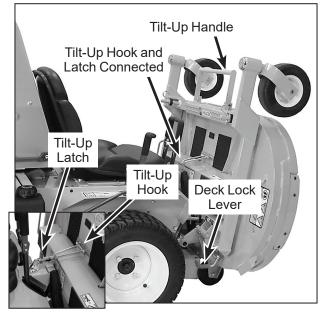
**Deck Secured in TILT-UP Position**
