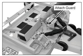
**PTO Shaft Guard Installation**
