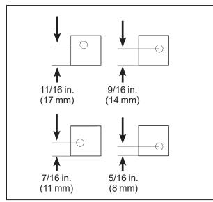
PTO Belt Tightener Stop Block Adjustments
