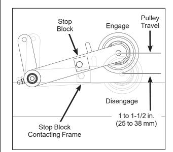
**Clutch Idler Pulley Travel Adjustment**
