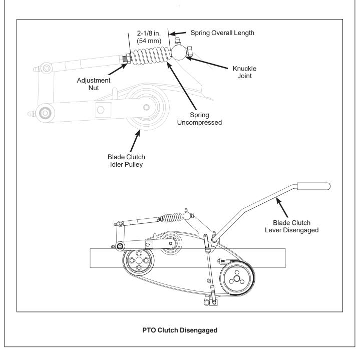
Use the following procedure to check and adjust clutch disengagement and brake action:
