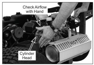
Check Cooling System Airflow
