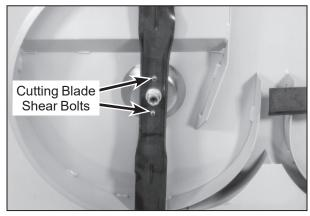
**Cutting Blade Shear Bolts**
