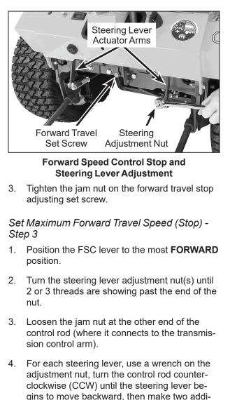
gins to move backward, then make two additional turns. Next, reverse and turn the control rod clockwise (CW) until the **steering lever stops moving forward** and then **make one additional turn.** Tighten the jam nut.
