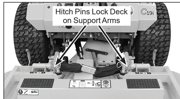
Use Hitch Pins to Lock Deck on Support Arms
