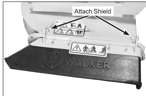
Discharge Shield Installation on Side Discharge Deck
