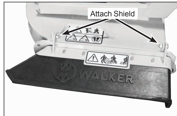
Discharge Shield Installation on Side Discharge Deck
