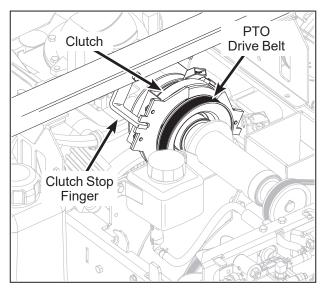
**Clutch Stop Finger in Locked Position**
