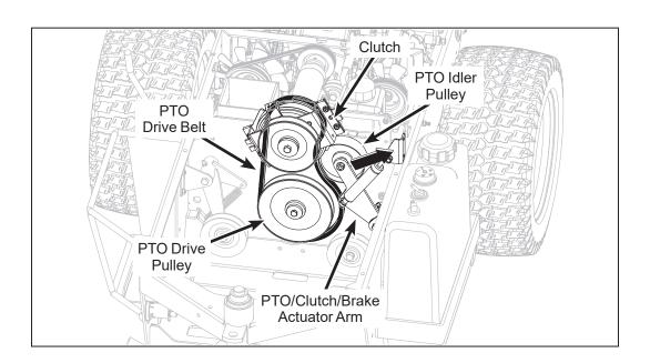
PTO Drive Belt (Disengaged)
