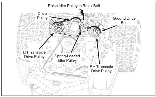
**Ground Drive Belt Assembly (Disengaged)**
