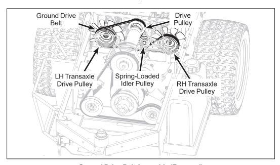
**Ground Drive Belt Assembly (Engaged)**
