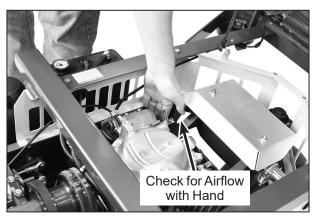
**Check Cooling System Airflow**
