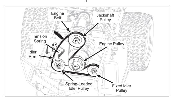
**Engine Belt (Disengaged)**
