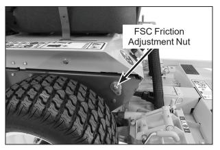
**FSC Friction Adjustment Nut**
