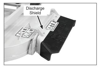
Side Discharge Deflector Shield in Lowest Position
