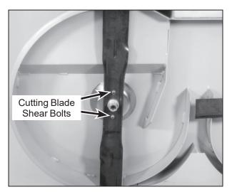
**Cutting Blade Shear Bolts**
