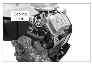
Inspect and Clean Cylinder Head Cooling Fins (Viewed from Right Rear Side of Engine)
