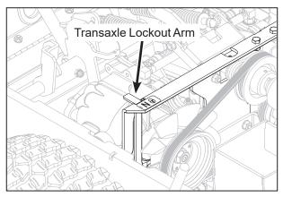
Transaxle Lockout Arm - Normal Operating Position
