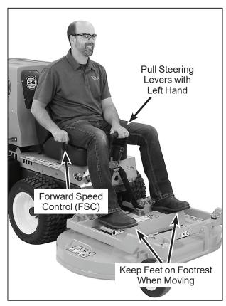
**Correct Operator Hand Position** on the Controls
