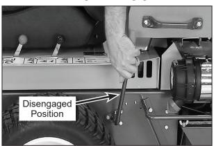
Parking Brake Disengaged
