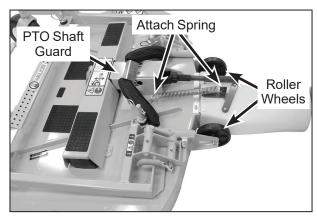
Tilt-Up Spring and Roller Wheel Installation on Collection Deck
