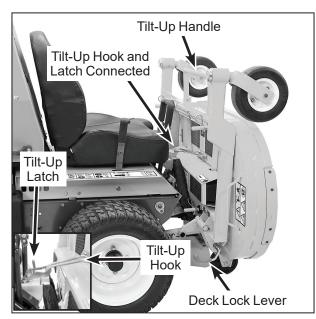
**Deck Secured in TILT-UP Position**
