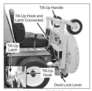
Deck Secured in TILT-UP Position
