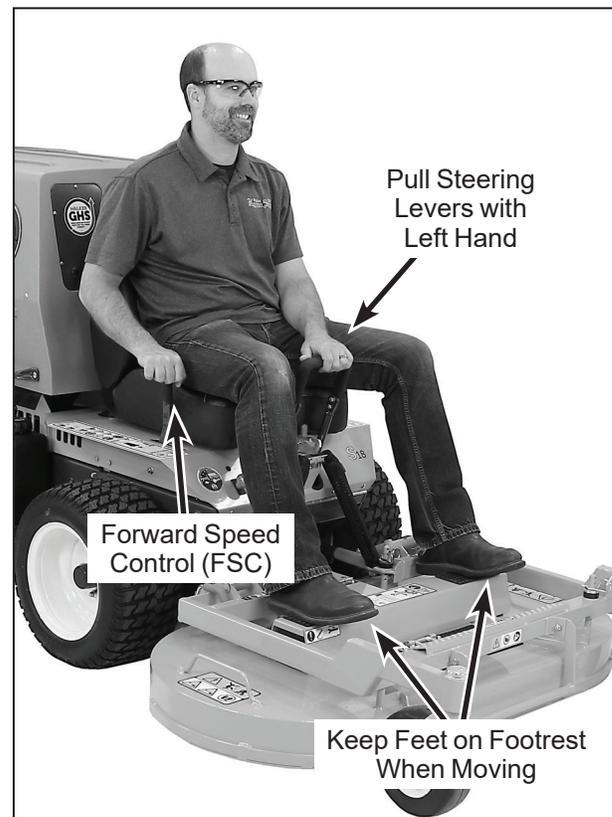
**Correct Operator Hand Position on the Controls**
