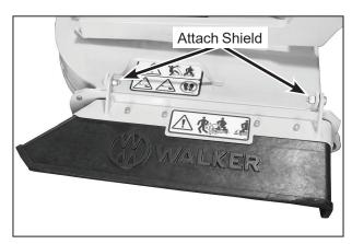
**Discharge Shield Installation** on Side Discharge Deck
