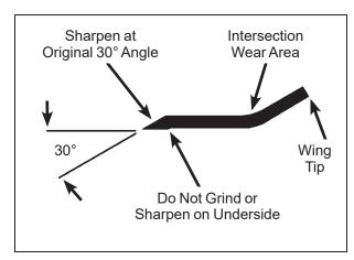
**Mower Blade Profile for Sharpening**
