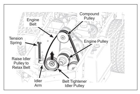
**Engine Belt (Disengaged)**
