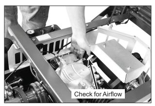
**Check Cooling System Airflow**
