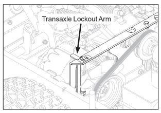
Transaxle Lockout Arm - Normal Operating Position
