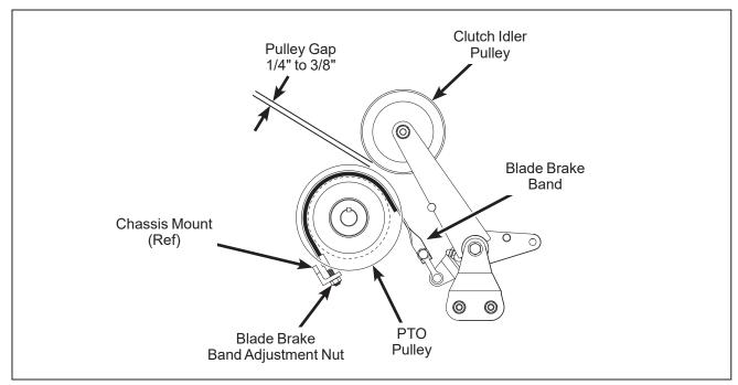
Blade Brake Band Adjustment (Clutch Disengaged)
