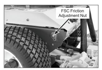
**FSC Friction Adjustment Nut**
