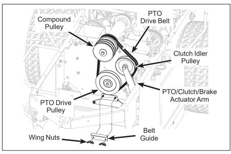
PTO Drive Belt (Disengaged)
