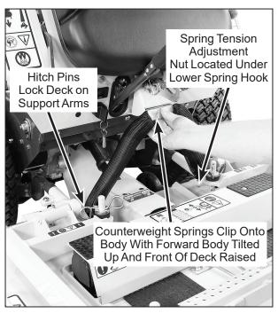
**Deck Counterweight Spring Installation**
