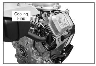
Inspect and Clean Cylinder Head Cooling Fins (Viewed from Right Rear Side of Engine)
