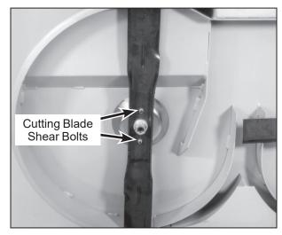
**Cutting Blade Shear Bolts**
