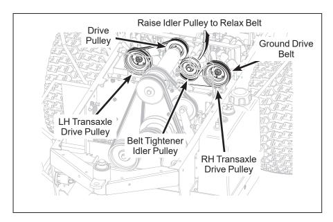
**Ground Drive Belt Assembly (Disengaged)**
