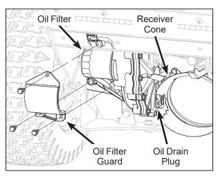
Transaxle Oil Drain Plug, Filter, and Guard Location
