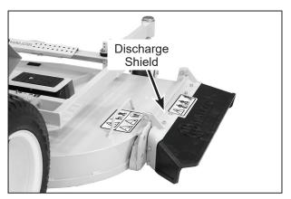
**Side Discharge Deflector Shield in Lowest Position**
