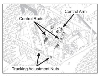
Transmission Control Rod and Arm Location (Shown with Parts Removed for Clarity)
