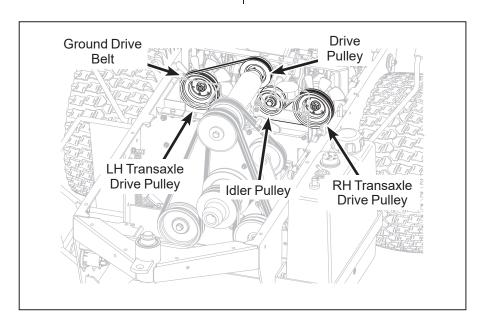
**Ground Drive Belt Assembly (Engaged)**
