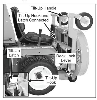
**Deck Secured in TILT-UP Position**
