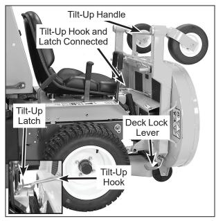
**Deck Secured in TILT-UP Position**
