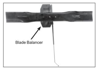
Blade Balanced on Magnetic Wall-Mounted Balancer
