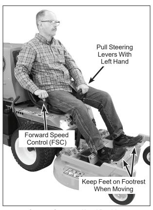
**Correct Operator Hand Position** on the Controls
